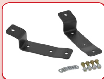
Dropped ARB Brackets
