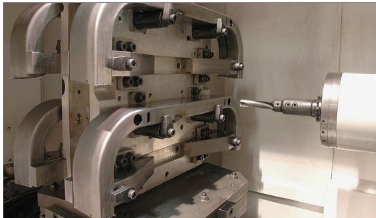
Locating features are machined into each crossmember to enable self-positioning of billet components.
