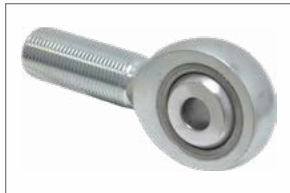
Includes 7/8"-shank x 1/2" bore, teflon-lined 4130 rod ends.
