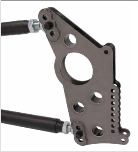
Doubler plates for 4-link mounting holes on both front and rear brackets. Axle brackets for 3", 3-1/4", or 3-1/2" tubes.
