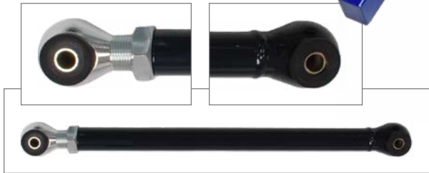
Adjustable length, poly-bushed rods ends
