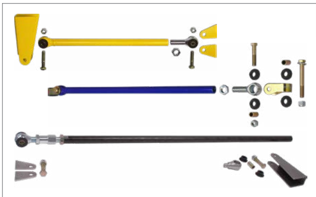
Bolt-on track locater or single- or double-adjustable panhard bar
