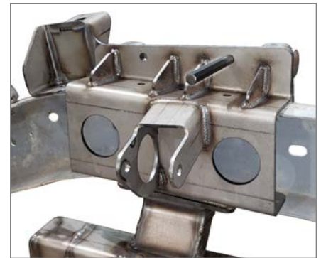
Engine mount assembly fully surrounds the frame and braces the control arm mounts.
