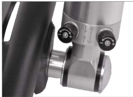
Gusseted lower shock mount with specialized hardware for more tire clearance.
