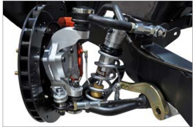
Adjusting the shock preload and dampening can be done without removing the shock.
