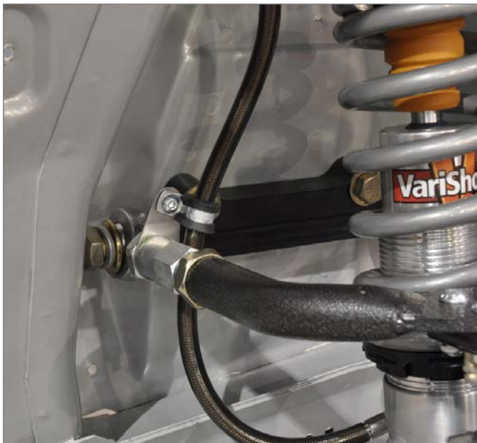
Various hardware is available to assist in safely routing the reservoir hose. The rubberized clamp and bracket set, shown above, fits against the jam nut of any 3/4" thread rod end or adjuster.
