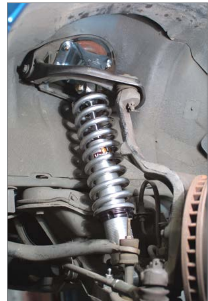
Coil-over kit includes springs, direct-fit upper shock mount and lower crossbar, upper spring seat, threaded locking lower spring collar, spanner wrench and mounting hardware.
