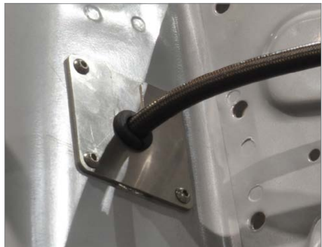
The passage bulkhead provides a clean and safe way of passing the remote reservoir through any accessible flat surface and secures the hose.
