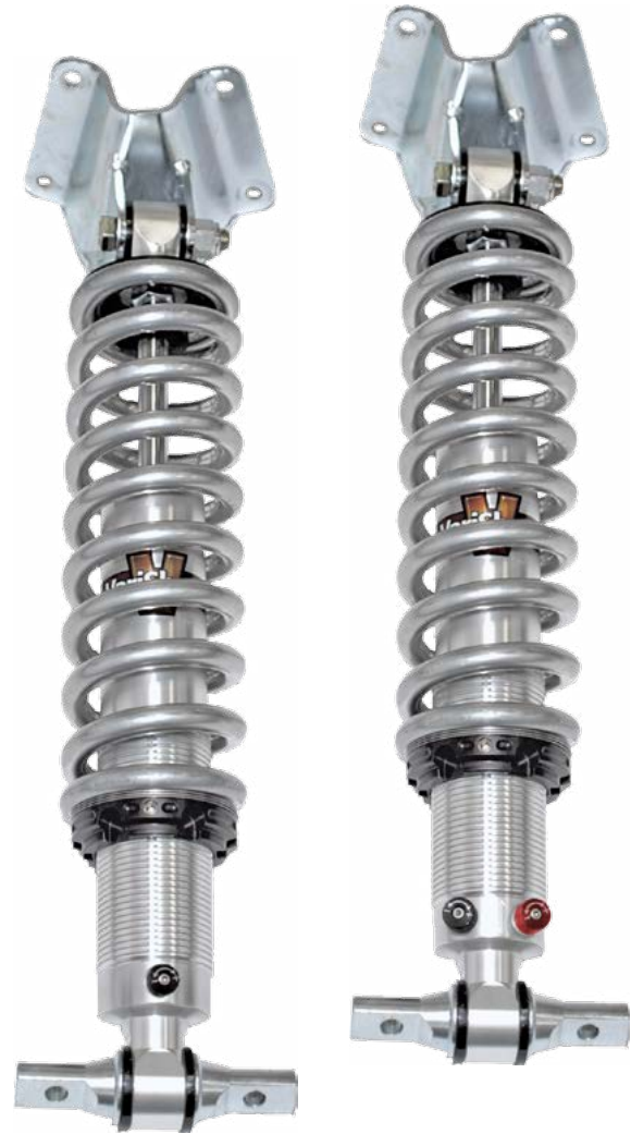
Coil-over kit includes springs, direct-fit upper shock mount and lower crossbar, upper spring seat, threaded locking lower spring collar, spanner wrench and mounting hardware.
