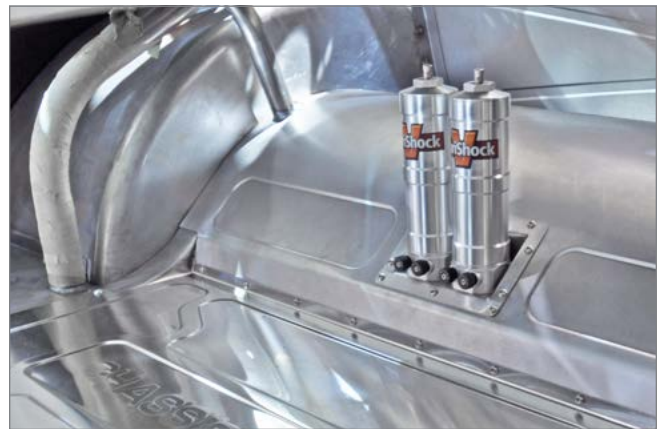
An optional shock mount inset is available with the trunk-area floor kit to cleanly display the reservoirs in the trunk.
