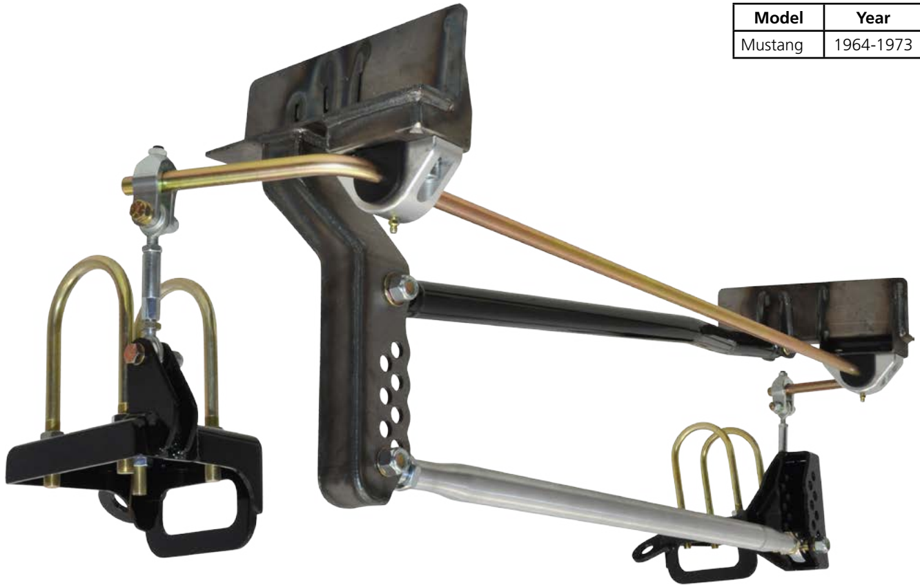
Shown with optional sliding-link anti-roll bar and driver-side spring plate.
