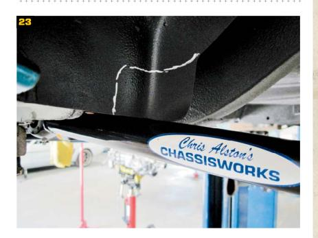
Here's the inside after welding and application of more Fusor seam sealer. When it comes to the brace that attaches the trunk hinge to the new mini-tub, you can either trim and re-use the original one or make a new one like we did.
