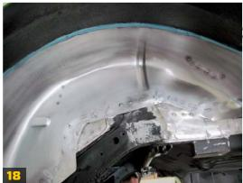
And here's how our closeout panels looked prior to welding. Notice how the predrilled holes in the panels line up with the framerail edges. This made doing the small rosettes even easier.
