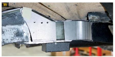
With the tub out of the way we could finish trimming away the metal. The best way to make sure you don't make the hole too big is to cut, test-fit the tub, then cut more if needed.
