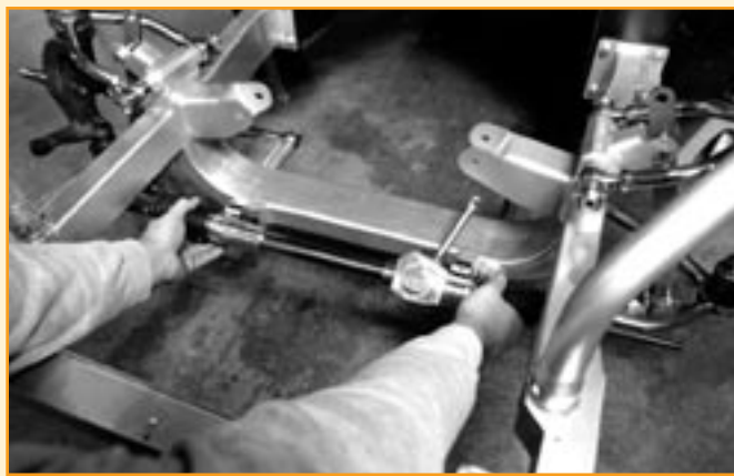
The rack assembly can be rotated in its mounts to provide the best angle for the steering-rack input shaft.
