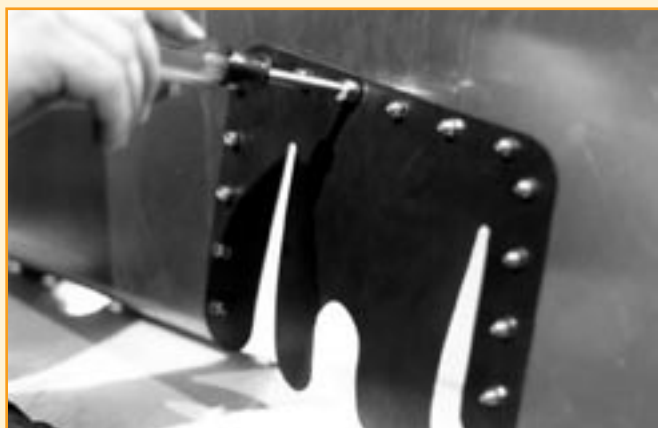
Our precut, rubber splash-panel boots are custom formed to fit around the suspension components; they are installed on the outer side of the panel.
