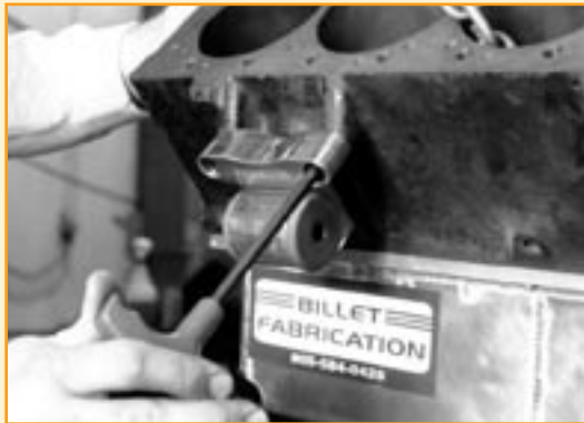
A steel sleeve rides inside the urethane bushings of our new, billet-aluminum motor mounts.
