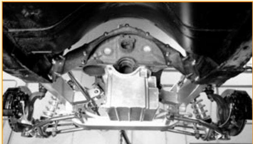
This shot from under the car shows another view of just about everything we've installed, plus the Wilwood brake calipers used with our rotors.
