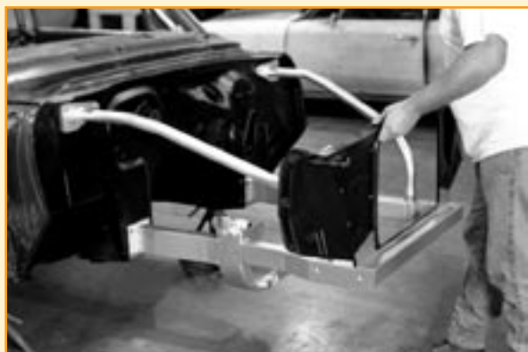
The radiator-core support simply slides in place behind the mounting tabs on each side of the front crossmember.
