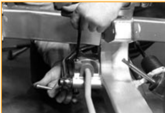
...and secured in place with the billet clamps.
