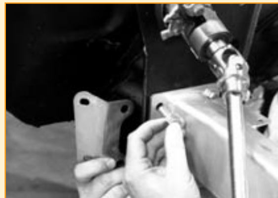
The brackets are attached to the back side of the frame mounts, using the two inner frame bolts on each side.
