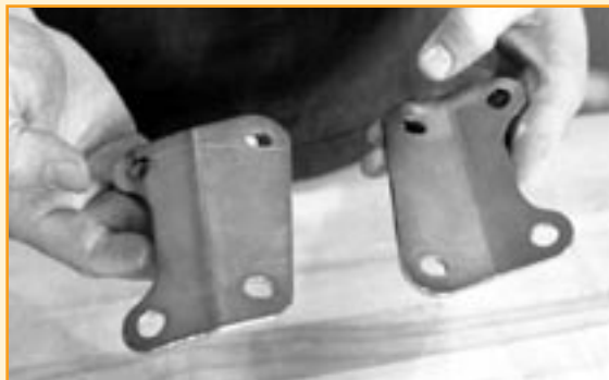
These mounting brackets are used to connect the midplate to the lower frame mounts.
