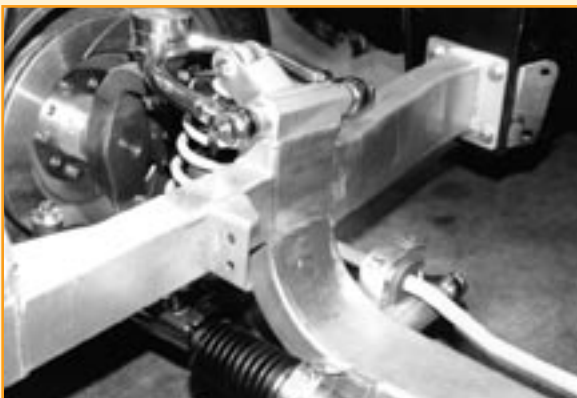
The bracket for attaching the motor plate to the frame can be seen just ahead of the crossmember. This bracket replaces the side-mount hardware, which is attached to the crossmember itself.
