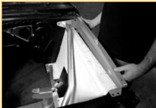
...and the fender/hood-hinge mount goes in next, under the splash panel and over the radiator-core support and upper strut mount.
