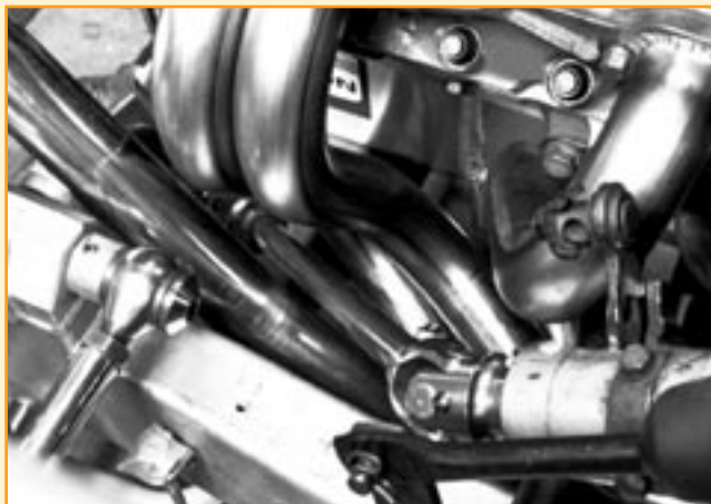
The view down the driver's side of the motor shows how the headers have been contoured to clear the steering linkage and frame...
