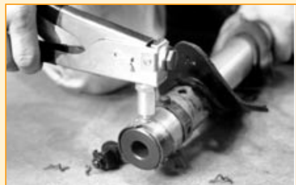
After holes are drilled into the end of the steering column, our bushing is installed flush with the end of the column and secured with blind rivets.
