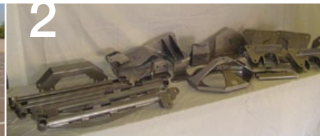
2 system producing 12 inches of travel. The system accommodates up to a 22-inch wheel, features a bolt-on Watts link to eliminate axle shift, and is designed for '63-87 GM trucks. The Porterbuilt Dropmember comes with the main X-member section, inner frame support plates, upper control arm/bag mount plate, transmission cross member, shock mounts, billet tie-rod ends and heavy duty Heim joints with hardware, aluminum shock mount bushings, C-notch for rack-and-pinion tie rod clearance, motor mounts, and all of the hardware and instructions.
