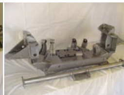
2 system producing 12 inches of travel. The system accommodates up to a 22-inch wheel, features a bolt-on Watts link to eliminate axle shift, and is designed for '63-87 GM trucks. The Porterbuilt Dropmember comes with the main X-member section, inner frame support plates, upper control arm/bag mount plate, transmission cross member, shock mounts, billet tie-rod ends and heavy duty Heim joints with hardware, aluminum shock mount bushings, C-notch for rack-and-pinion tie rod clearance, motor mounts, and all of the hardware and instructions.
