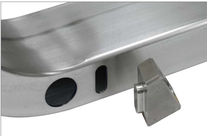
Billet rack-and-pinion mount inserts into machined crossmember slot.
