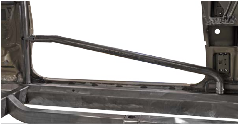
Quick-Release L-Handle Pin Push-button ball-lock pin available for quick removal of door bar and back brace.
