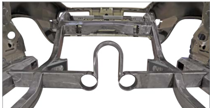
Tall driveshaft loop allows body to sit lower over the drivetrain without risk of driveshaft contact. Crossmember features factory-welded, dual 4"-ID exhaust ports.
