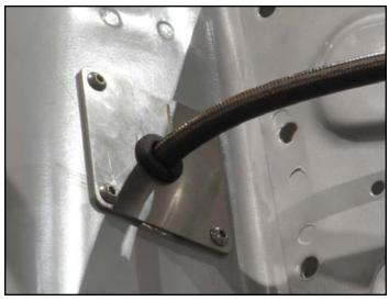
The passage bulkhead provides a clean and safe way of passing the remote reservoir through any accessible flat surface and securing the hose.
