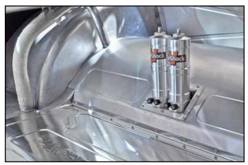
An optional shock mount inset is available with the trunkarea floor kit to cleanly display the reservoirs in the trunk.
