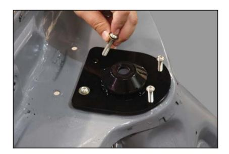
22. Install the flat washer and locknuts on the two outer bolts and tighten to hold the mount plate securely.
