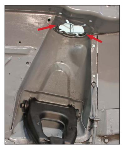
13. Use a disc sander to remove the two lips as shown.
