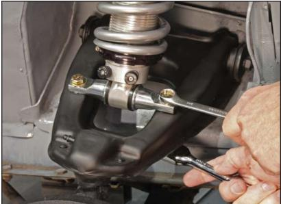
39. The coil-over shock and spring are now installed.
