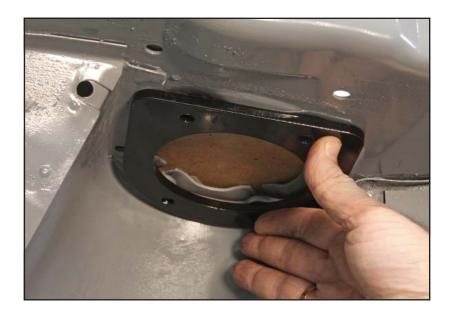
The upper shock towers are sightly different on the 1962-65 and 1966-67 models. The 1962-65 is shown on the left and will need the modifications in steps 17-20 before the upper coil-over mount plate can be installed. If you are working on a 1966-67 model, skip to page 11.
