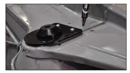
18. Use a disc sander to grind the lip until the plate sits flat on the tower.
