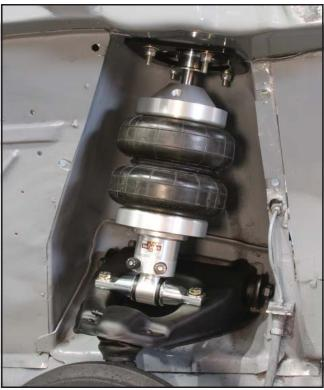
• The Air spring is larger in diameter than the coil-over. When reinstalling the bumpstop plate you will need to shim it out with washers. There must be at least 3/4" of clearance between the bump-stop plate and the air spring. If the air spring rubs on the plate during travel it will be damaged and this is not covered under the warranty in any way.
