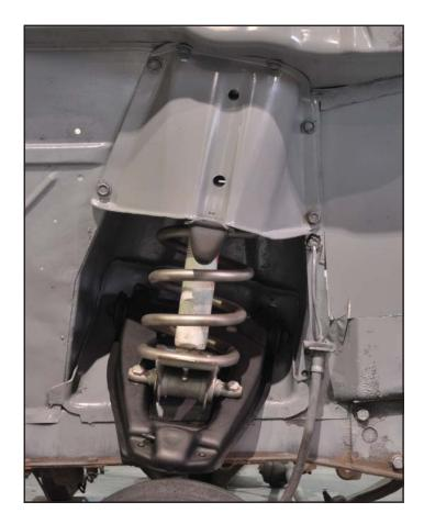
5. The upper shock mount is attached to the shock tower. It will be removed and replaced with the coil over mount.
