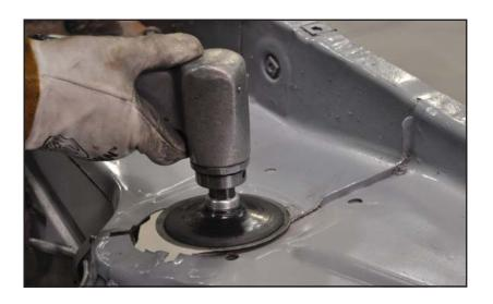
19. The plate now fits correctly and is ready to be installed.
