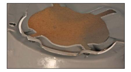
15. Trial fit the shock tower backup plate (210142), sand the lips until the plate fits tight.
