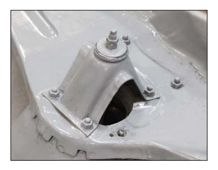
6. Unbolt the upper shock mount from the shock tower and remove the nut, washer, and bushing from the shock stem.
