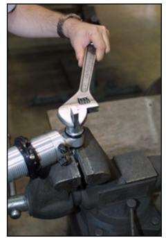
Installing lower crossbar and urethane bushings.
