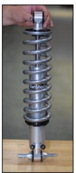
Coil-over and spring assembly ready to install.
