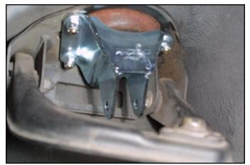
Upper shock mount is bolted into position.
