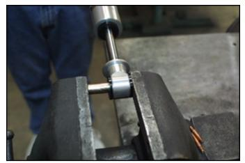
Installing upper urethane bushings and steel sleeve.
