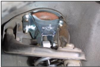
Upper mount with coil-over assembly bolted in.
