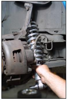
Installing the coil-over assembly.
