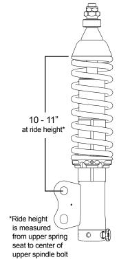
to correct any major vehicle ride height issues. It may take some work with spring rates and upper mount relocation to get the correct combination of vehicle ride height and front suspension travel for your application.
