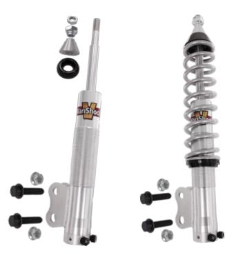
**Description:** Bolt-on strut directly replaces factory strut in 1982-1992 Camaro and can be used with coil spring in stock location. Additional components included with VAS 872DP-952 enable removal of factory positioned coil spring for conversion to 2-1/2" coil-over spring.
