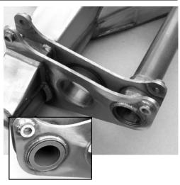
^ The drag anti-roll bar mounts directly through an integrated tube attached to the underside of the FAB9, and rotates in low-friction bushings (inset). The bar itself is 1.25-inch diameter steel, while the end links are billet aluminum, and the two are joined via a 48-spline connection on the ends. Adjustable end links tie into weld-on mounts on the frame via spherical bearings on each end. You'll also note that the anti-roll bar mount is equipped with the optional wheelie bar mounting points.
