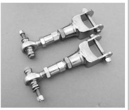
A Everybody and their brother makes adjustable upper control arms; what sets Chassisworks apart is that they offer both a "competition" version rated up to 800 horsepower, with the beefier Pro Power units like ours made of even stouter materials and components for pro-level drag race applications.
