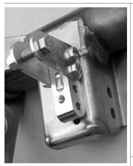
↑ Stock-style shock mounts are standard, but the flanges on the FAB9 are drilled with four holes to allow a 1.75-inch range of ride height adjustment. If you need even more, Chassisworks' adjustable coilover mounts add another four holes, plus the side brackets can be flipped as well to allow up to 2 5/8-inch adjustment in 7/16-inch increments.
