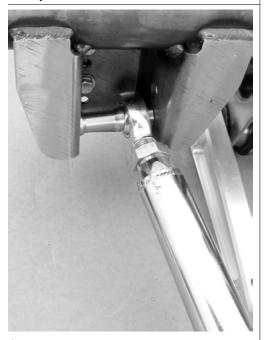
↑ The FAB9 is designed to accommodate any stockstyle lower control arm, and has two sets of mounting holes, with one in the stock position and one relocated down by 1.125-inches to allow adjustment of the suspension geometry. When combined with the offset spacers on the Pro Power lower control arms, you end up with a ton of extra inboard tire clearance.
