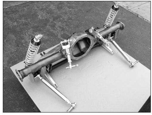
since we're not planning on taking the Panda out on Date Night, we went for the spherical bearing setup for increased precision. Beyond the choice of width and upper control arm mounting, you can also specify additional back bracing, an integrated anti-roll bar mount, built-in wheelie bar mounting points, and inboard coilover mounts. With the exception of the latter option, we checked all the boxes and ended up with the gorgeous piece you see here.
