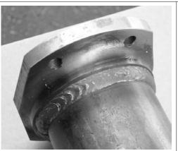
A It's possible to order a FAB9 with bare ends, or with the ends unattached to allow you to trim the tubes yourself, but Chassisworks does a very, very nice job putting them on if you let them. The FAB9 comes with Torino-style housing ends to allow for large-diameter axle shafts, and brake systems designed for "Late Ford" ends are a direct bolt-on to the billet flanges.
