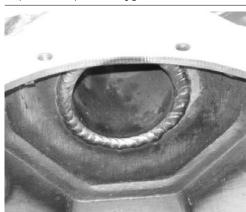
^ The strength of our FAB9 is obvious from the first glance, but one thing you won't see when it's all buttoned up is the fact that the 3-inch axle tubes are welded both externally where they meet the fabricated steel center section, but internally as well at the center bulkhead, giving two widely-spaced points of support for each tube. It's details like this that make the FAB9 a standout.
