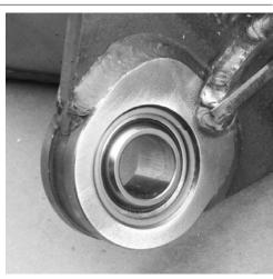
A The FAB9 is available with provisions for polyurethane bushings at the upper control arm mount, or spherical bearings like our axle housing. The bearings are replaceable, and are retained with a spiral wire lock.
