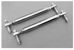
Like the uppers, the Pro Power lower control arms are double-adjustable for length without having to remove an end, to make squaring the axle to the chassis a simple process.
