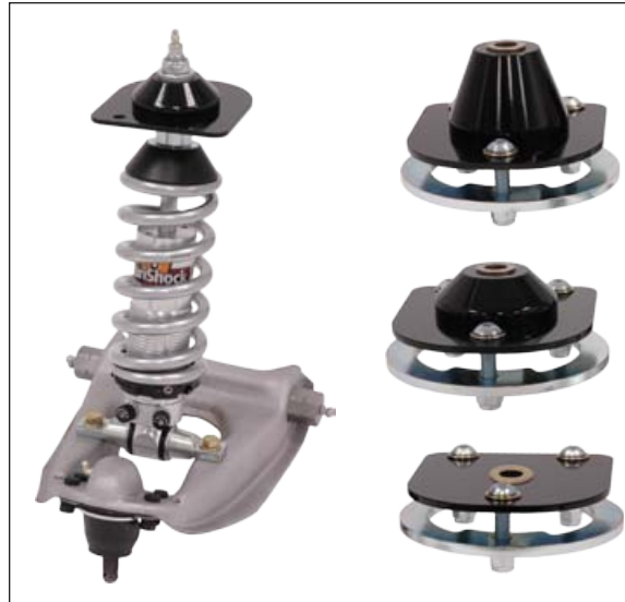
This style of shock mount adapter, used on early Mustangs and Chevy IIs, bolts directly to the factory shock towers and allows the shock's pivot-ball stud to be mounted at different positions to vary the ride-height adjustment range.
