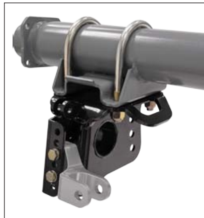
Bolt-on shock mount adapter for GM leaf-spring pad
