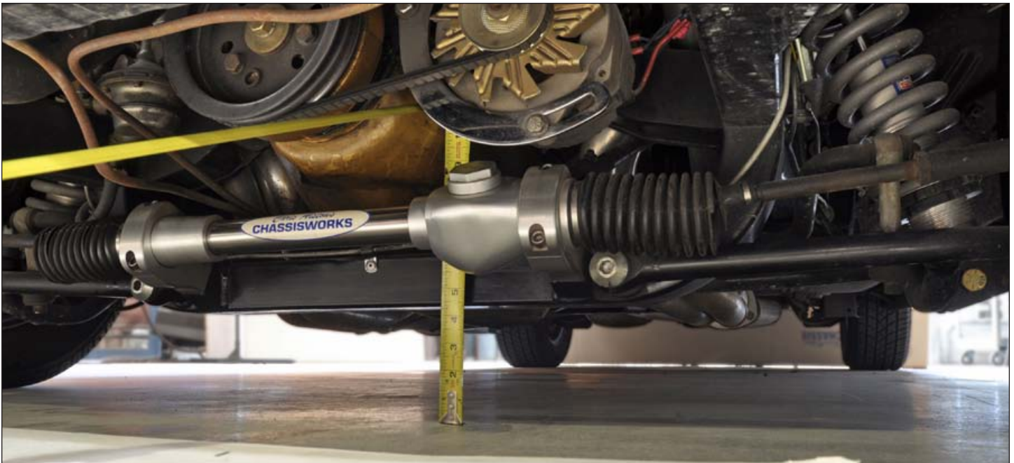
Chassisworks measures vehicle ground clearance from the bottom of the suspension crossmember directly to the ground.
