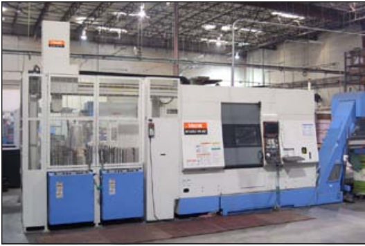
One of the multiple fully-automated machining centers that Chassisworks utilizes to manufacture the precision components required for VariShock and various private label shock absorber brands.
