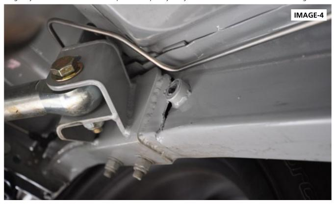
Image-5 - This view from our instruction sheet shows the proper bolted installation of the support tab for upper control arm front bracket where it connects to the chassis.
