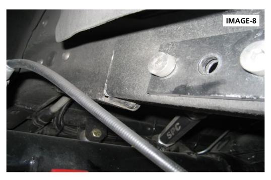
loads to the system cradle beyond its original intent. Additionally, the u-bolts that attach the cradle to the stock frame have not been installed, requiring the welds to carry all the loads.
