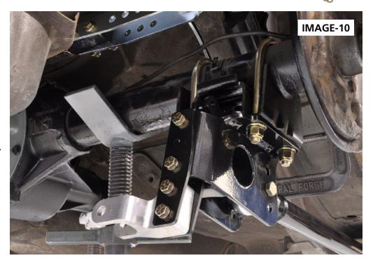
bind the suspension links. If the 2-1/2" reduction is too low, flip the lower mounts over and the car will only sit 1-1/4" lower. You may be able to actually drive the car with the 1-1/4" reduction in bump travel, but the shock brackets lowest edge will be below bottom of an 18 inch diameter rim so the ground clearance is way too little to drive it like this on a public road.
