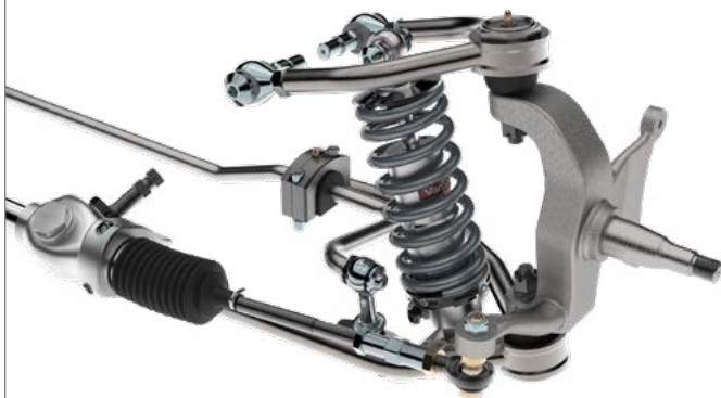
5762 STREET MACHINE ARMS WITH SCULPTED SPINDLE, MULTIPLE BRAKE OPTIONS
