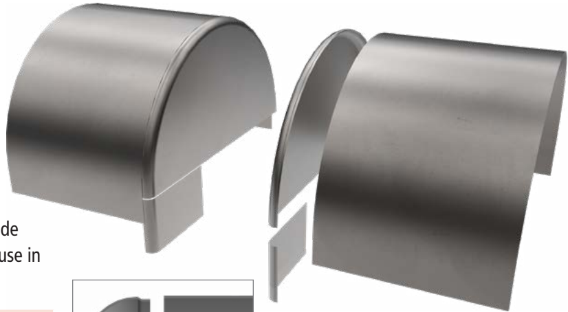
Offset tub-cap lip seats underneath edge of tub skin, creating an easy to align overlap joint with flush outer surface.
