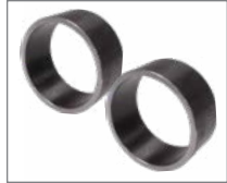
Crossmember exhaust ports; not installed.
