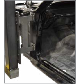
A-pillar (hinge bosses) body adapter
