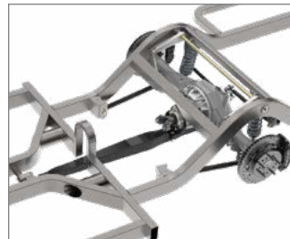
Torque-Arm Watts Link More emphasis on cornering and acceleration performance
