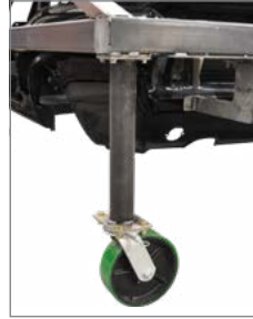
Rear caster with extended fixture legs
