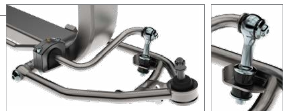
Crossmember-mounted bushing housing; poly-bushing lower end link
