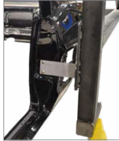
B-pillar (door striker) body adapter
