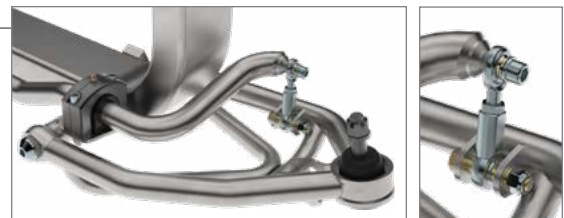
Crossmember-mounted bushing housing; poly or COM-8 lower end link
