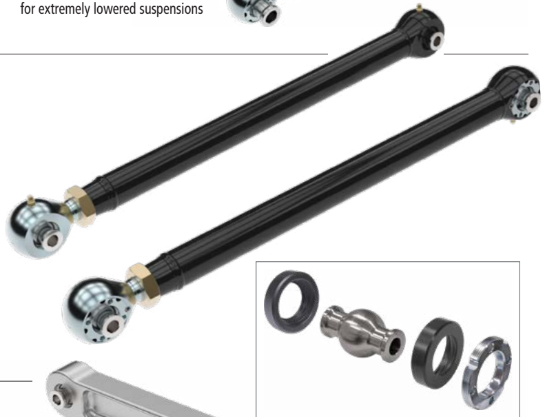
Double-Adjustable Arms Broader adjustment range required for extremely lowered suspensions
