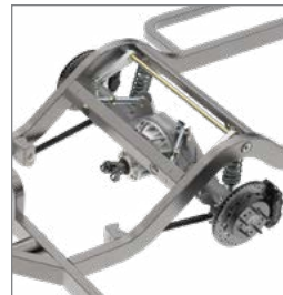
Canted 4-Link Well-rounded system for street and handling performance
