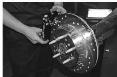
This is followed with the installation of the actual Wilwood four-piston disc brake calipers using the provided mounting brackets using 3/8-24 nuts and bolts. And that's all for now, gang!
