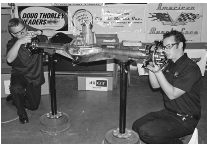
Then Bret and Dan tighten down the axle bearing retainers side-to-side.
