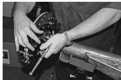
This is followed with the installation of the actual Wilwood four-piston disc brake calipers using the provided mounting brackets using 3/8-24 nuts and bolts. And that's all for now, gang!
