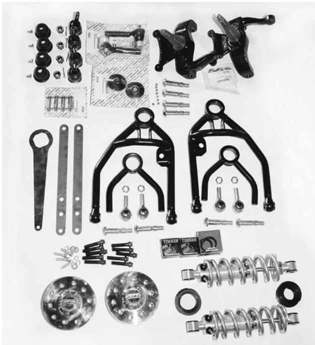
This parts layout photo shows the entire Chassisworks un-equal length, upper and lower a-arm suspension system including A-arms, ball joints, a ball joint wrench, set of Chassisworks dropped front spindles, bushings, mounting hardware, a pair of shock absorbers, Alston VariShock, double adjustable coil-over shocks, and Chassisworks front hubs.
