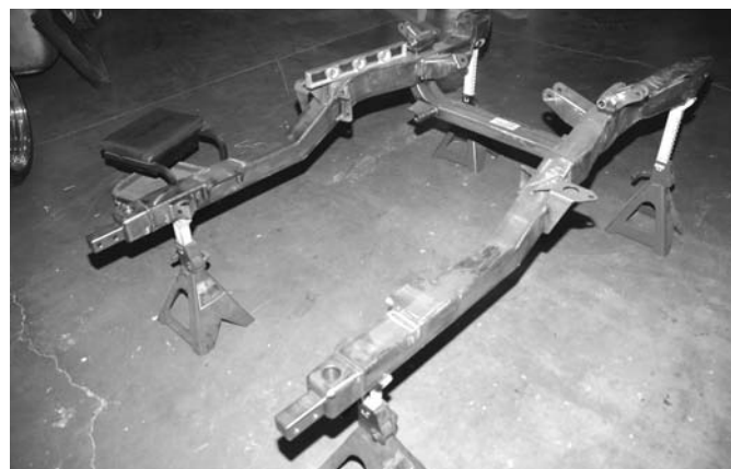
This is our bare Chris Alston Chassisworks 1967 to 1969 front clip, or sub frame (p/n 917701) leveled out on a set of jack stands to insure that all suspension components are correctly aligned upon assembly. These sub frames are manufactured out of CNC die stamped and laser cut boxed steel which is welded together to form a rock-solid foundation. This setup also features a trick mandrel bent 2x4-inch front cross member, and all suspension and engine mount brackets are CNC machined. Alston's front sub frame even comes with its own alignment pins to make installation hassle free.
