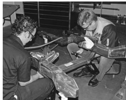
With all the threads cleaned and chased actual lower control arm assembly begins using the special 7/8-inch Allen head pivot studs provided.
