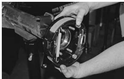
Next comes the installation of the Wilwood-Ford emergency brake assemblies which are mounted up to the Fab-9 axle bearing flanges using four, (4) 3/8-inch retaining nuts and bolts.
