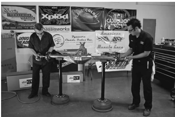
Next comes the installation of the Wilwood-Ford emergency brake assemblies which are mounted up to the Fab-9 axle bearing flanges using four, (4) 3/8-inch retaining nuts and bolts.
