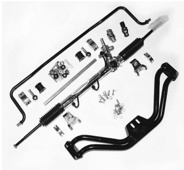
And there's more. In this second parts photo, we see the remainder of the Chassisworks frame assembly (there's a lot of stuff here, folks,) which includes the front anti-sway bar, a polished Chassisworks power steering rack, and Chassisworks tubular front transmission cross member setup for a Tremec TKO 500 five-speed transmission.
