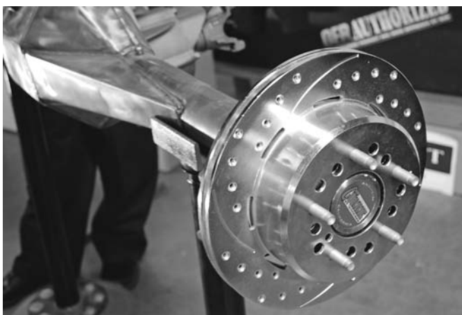
On go the Wilwood Brakes 12.19-inch slotted and cross drilled rotor's or rear "hats."
