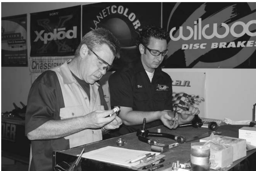
Actual suspension component assembly begins with Maxwell chasing threads on the control arms, while Dan Woods follows up with a little anti-sieze to the control arm adjusters for ease in installation. This procedure is followed with the installation of the actual ball joints themselves using the provided ball joint installation tool.
