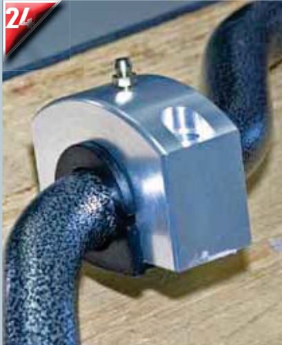
24 TCP provides these billet sway bar bushing mounts, which give solid integrity along with good looks.
