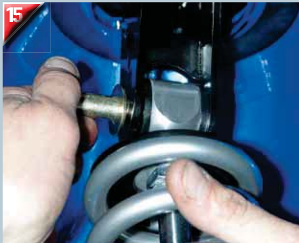
15 The top mount is secured on both sides with these nice cad-plated bolts provided by TCP.
