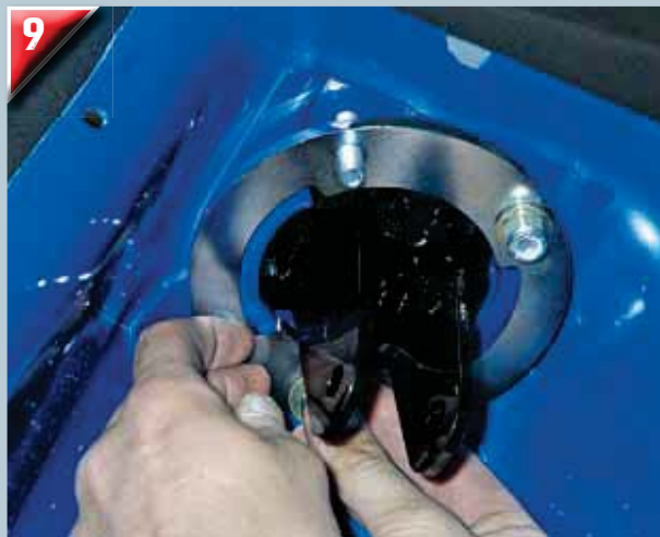
9 Install the coilover shock mount retaining plates and locknuts in each tower.
