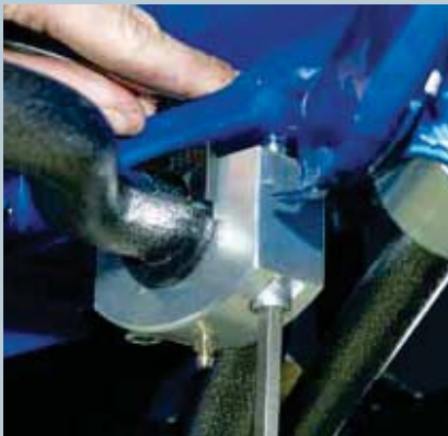
25 Richard secures the Mustangs Plus Grab-A-Trak hammered-metal sway bar at the same attachment points as stock.
