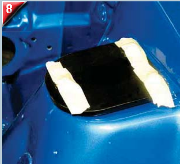
8 Use masking tape to hold the retaining bolts. You will need to install the retainer plate and locknuts underneath.
