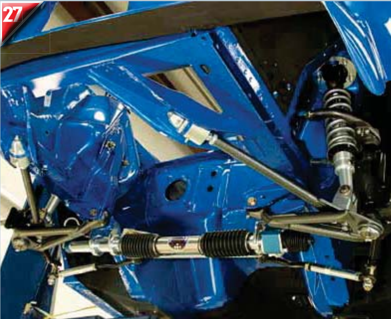
27 Our TCP/Grab-A-Trak front suspension is good to go. Reclaim gets TCP's newest suspension trick for classic Mustangs. ●
