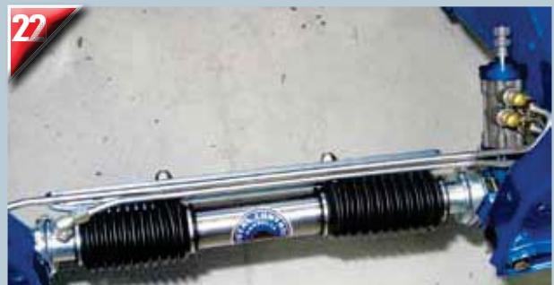
22 This is the installed TCP power-steering rack—a clean installation designed to clear just about anything. It will dramatically improve steering and handling.
