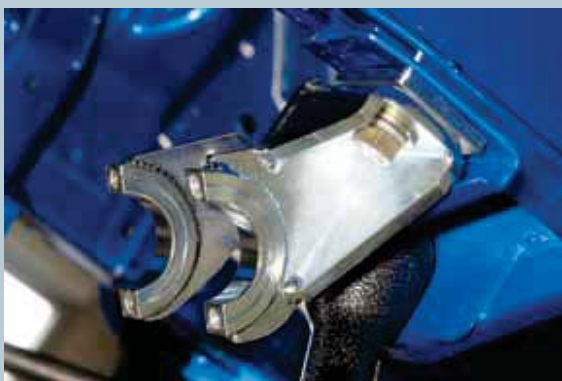
18 TCP's power rack-and-pinion steering installation begins with end brackets, which attach as shown using lower control arm pivot bolts. They also attach with crossmember mount bolt holes.
