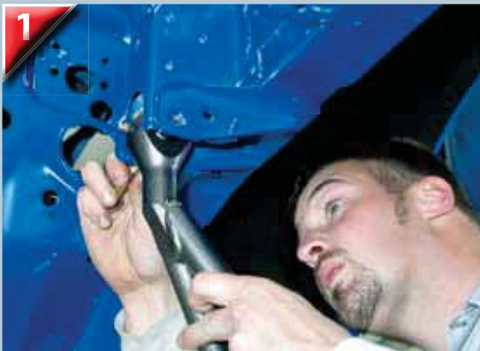
1 After methodical detailing and inspection, Richard Bramlett begins work installing our TCP front suspension. Heim joints have been lubricated with chassis lube and are good to go. Lower control arms go in first.
