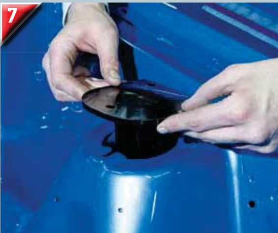
7 Position the upper coilover shock mount. Be careful if you have fresh paint like Project Reclaim.
