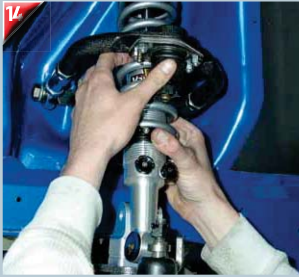
14 The coilover VariShocks are installed next, mounted at the top of the shock tower, then tied to the lower control arm.
