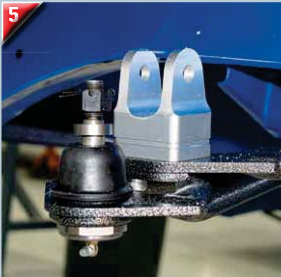
5 This is how the bottom billet coilover shock mount installs, fastened with strut rod bolts.
