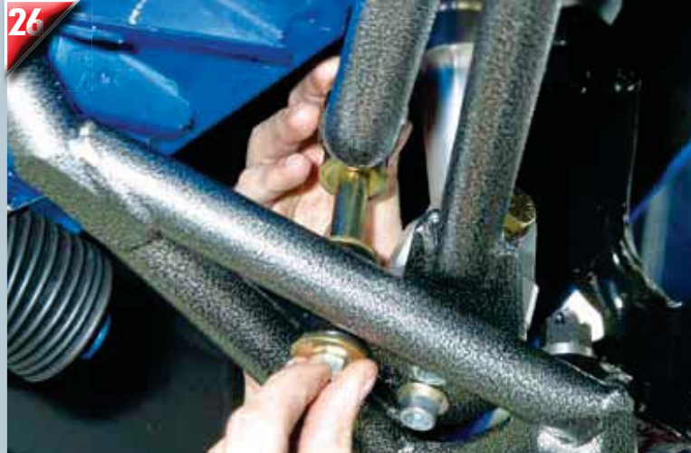
26 Urethane stabilizer links are next, installed with generous amounts of lubrication to eliminate squeaks and other noises. You have a choice of urethane or polyurethane. Urethane is rock hard, while polyurethane is more flexible and quieter. Remember: The bolt-head goes on top, not bottom.
