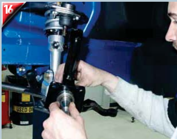
16 Richard installs the spindle provided by Mustangs Plus. This is a heavy-duty, '70-and-up Mustang/Maverick/Granada spindle.
