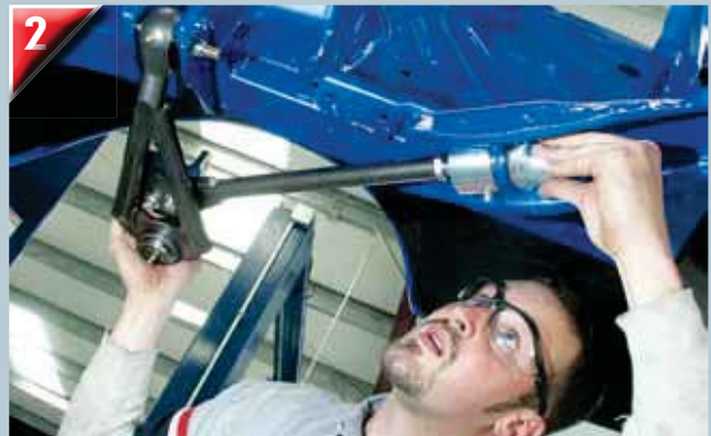
2 Fully articulating strut rods are next. Instead of the crude bushings Ford used, TCP has this nylon wrapped in an aluminum ball-socket arrangement. It stays adjusted and moves smoothly with the suspension, taking the "klunk" out of the bumps and keeps you on course.
