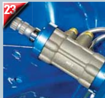
23 Power rack-and-pinion works the same way as worm-and-sector power steering by putting hydraulic pressure to work to assist steering efforts. Steering input runs this spool valve back and forth, which directs fluid pressure to one side of the ram or the other. The nice thing about TCP's power rack-and-pinion is how little space it consumes—and the power it provides.
