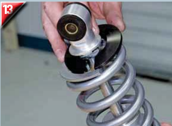
13 This is the spring retainer, which inserts on top. The bottom spring seat adjuster is modified once the Mustang is on the ground. That's when you adjust ride height using a tape measure. Don't change ride height until the vehicle is completely assembled.
