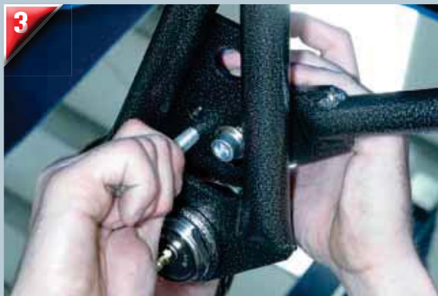
Here's how the strut rod and lower control arm tie together. Richard stresses following TCP's instructions, torquing all fasteners to specifications.
