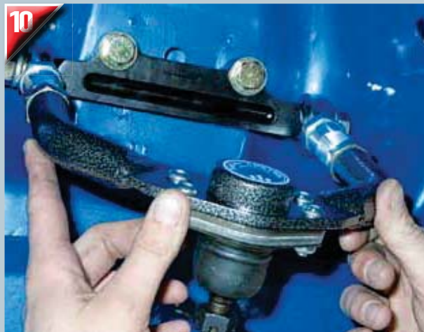
10 TCP upper control arms are next. Because we're using coilover shocks, there's no control arm spring perch to install.
