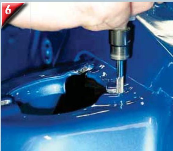
6 Be prepared to alter shock tower mounting holes in order to install upper coilover shock mounts.
