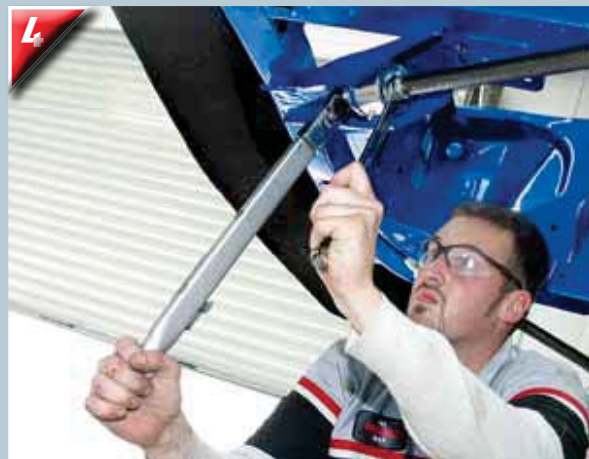
Richard uses a torque wrench and lubrication on every fastener.
