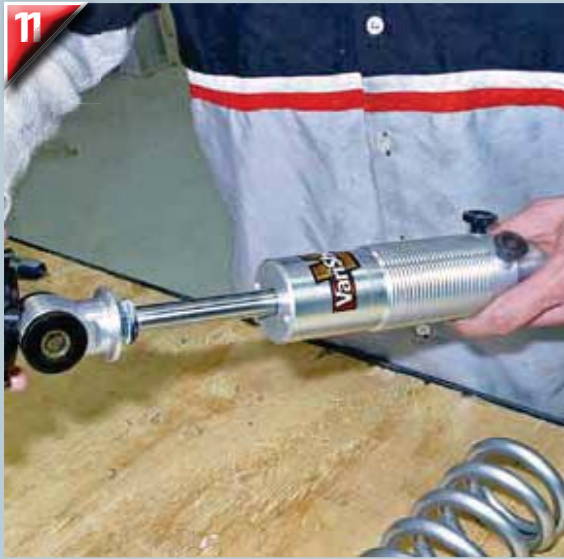
11 Coilover shock assembly is easy, beginning with spring adjusters, which screw on like this. This is an adjuster and a spring seat.
