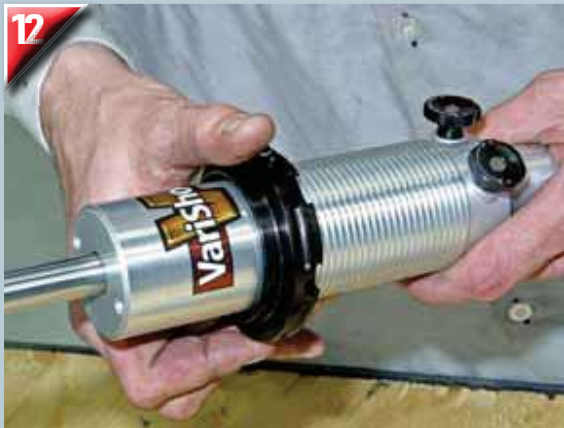
12 The VariShock shocks are adjustable three ways. There are two dampening adjustments—one for up and one for down. Adjust your ride and handling accordingly. Just reach inside the wheel-well and make finite adjustments. Coil spring adjustment controls ride height; run spring retainers up or down to adjust it.
