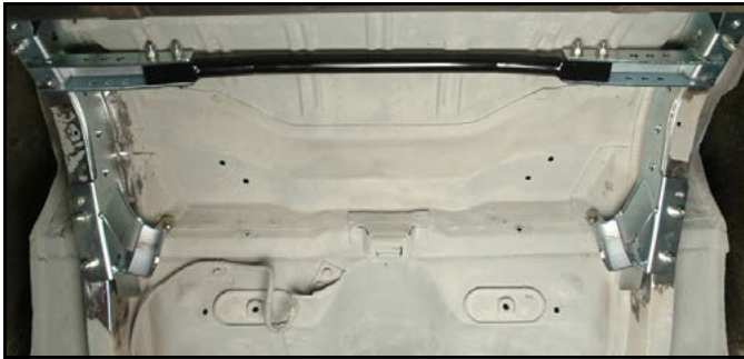
Camaro/Nova installation relies upon the frame rail and the vertical panel of the body to correctly position the suspension cradle.
