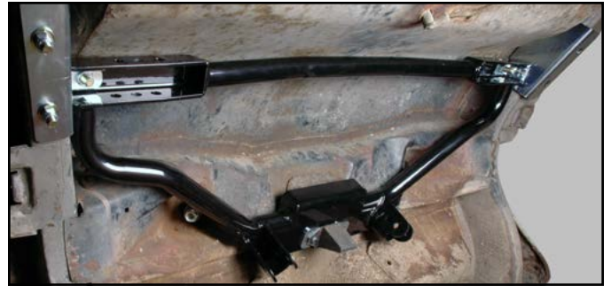
Mustang/Cougar installation utilizes existing pinion snubber and top shock mount factory bolt holes to locate the suspension cradle.
