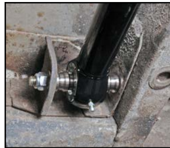
Lower links bolt directly in place of the factory leaf springs; all hardware included.
