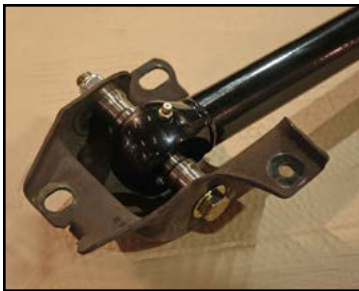
The lower link bolts into the factory leaf-spring bracket before installing onto car.
