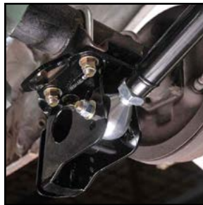
OEM mounting studs are replaced with supplied Grade 8 U-bolts.
