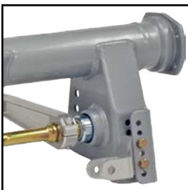
Splined-end anti-roll bar
