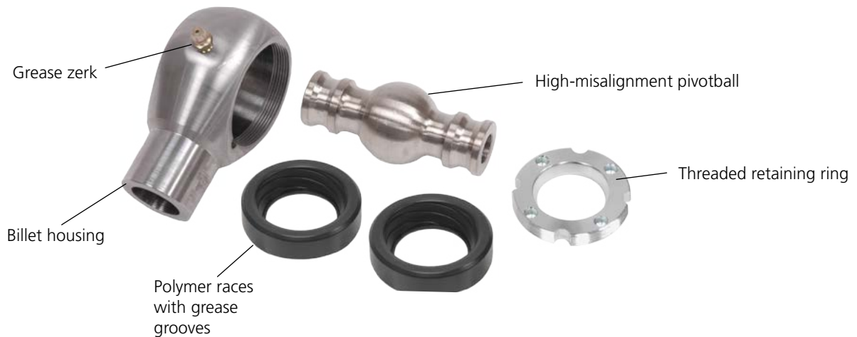
Centered Pivotball for stock wheel tub configuration.
