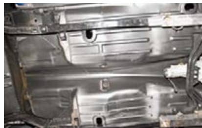
With sub frame connectors properly bolted up, they should butt up to the Chassisworks front sub frame like this.
