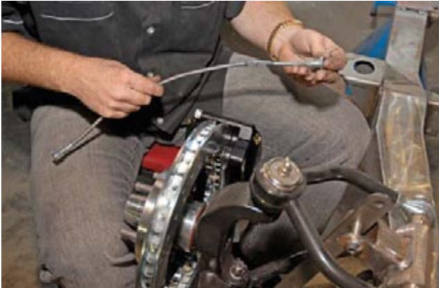
With that done, we see the installation of the provided 3/8-inch, braided stainless brake lines.
