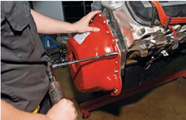
After installing the SACHS clutch and pressure plate, Bret Maxwell bolts up the Lakewood big-block bell housing using the mounting bolts provided with the bell housing. CHOP, CUT & REBUILD host Dan Woods provides a little assistance.
