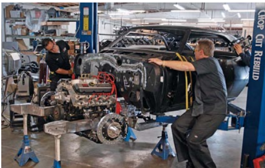
Prior to dropping our 502 big-block power train into place, Woods and Maxwell install the Chassisworks transmission cross member using the provided bolts in the Chassisworks kit.
