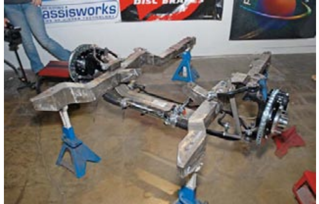
Shown is the 90% completed Alston Chassisworks front frame.
