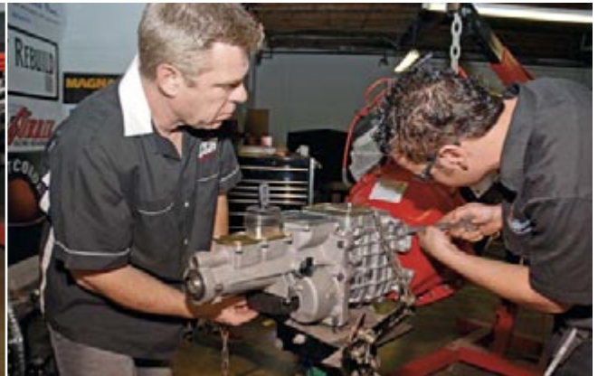
After installing the SACHS clutch and pressure plate, Bret Maxwell bolts up the Lakewood big-block bell housing using the mounting bolts provided with the bell housing. CHOP, CUT & REBUILD host Dan Woods provides a little assistance.
