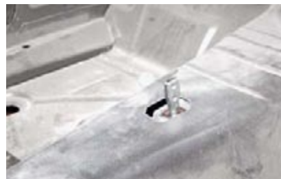
Next, Maxwell and company measure straight up from the shifter location of the TKO 600 transmission, and cut a "shifter slot" measuring approximately 1-1/2 x 3-inches in the center of the transmission tunnel.
