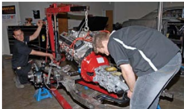
At this juncture it's time to begin positioning the big-block and five-speed into the Alston chassis.
