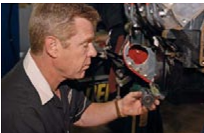
Next, our man Dan installs the Chassisworks motor mounts provided using the provided 3/8-16 x 1-1/2-inch socket head Allens and 3/8-inch washers provided.
