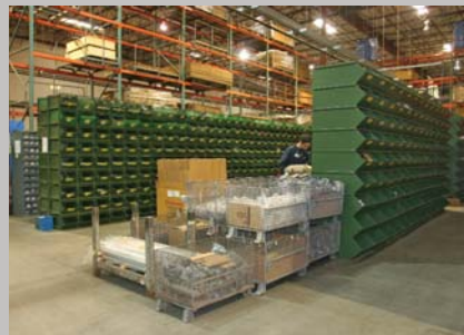
With the volume of product Chassisworks/KP pumps out they need to be organized, and they are. Rows of bins containing hardware for specific suspension kits allow product builders to quickly and efficiently obtain the parts needed to construct a given part.
