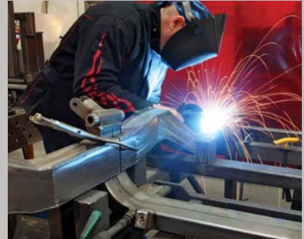
A front sub frame is loaded into the jig for final welding. The sub frame is held firmly in the jig with hardware so that none of the rails can move while they are being permanently joined together; this ensures the precise geometry of the clip is maintained.
