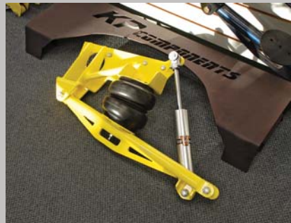
Here you can see some of the steps involved in producing the well-known KP Components cantilever setup. First, the metal is cut and bent to spec, then each kit is welded together and inspected before being sent out for powder coating and shipping.
