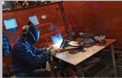
A front sub frame is loaded into the jig for final welding. The sub frame is held firmly in the jig with hardware so that none of the rails can move while they are being permanently joined together; this ensures the precise geometry of the clip is maintained.
