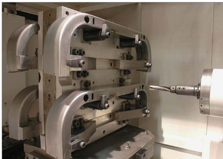
Locating features are machined into each crossmember to enable self-positioning of billet components.
