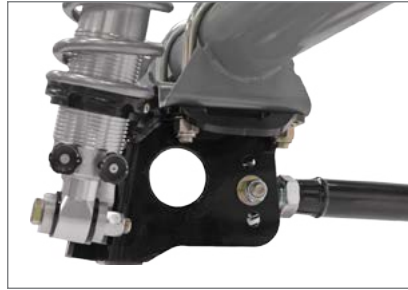
Multiple-position FAB9 lower arm bracket
