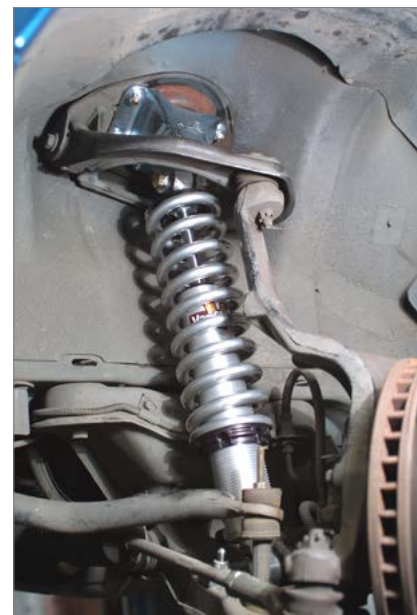
Coil-over kit includes springs, direct-fit upper shock mount and lower crossbar, upper spring seat, threaded locking lower spring collar, and mounting hardware.
