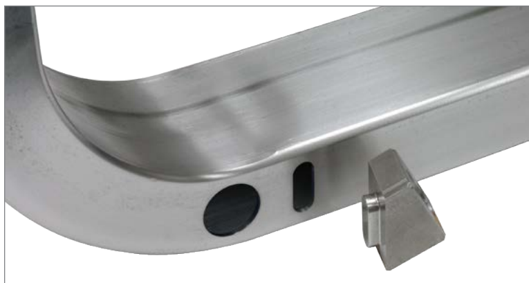
Billet rack-and-pinion mount inserts into machined slot on crossmember.
