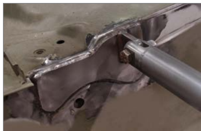
Firewall Mount Plate shown with standard bolt.
