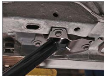
Lower links mount at OEM leaf-spring brackets
