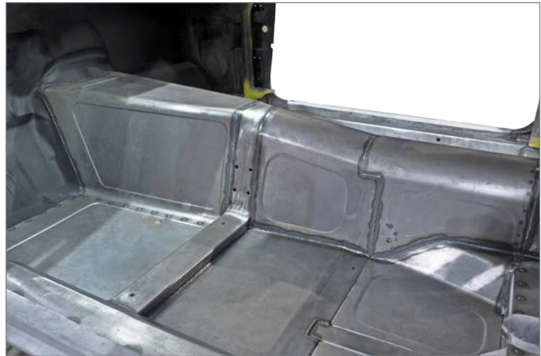
Installed lowered-seat-mount assembly shown with prefabricated front floor, transmission tunnel, driveshaft tunnel, and rear floor.
