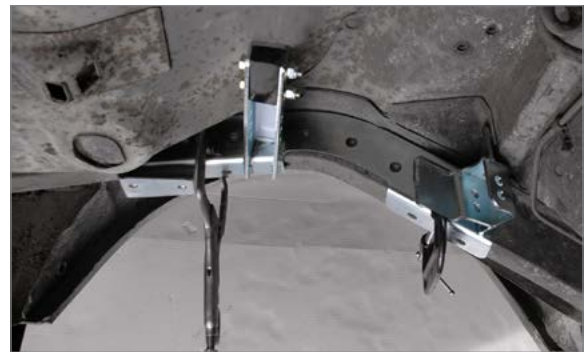
"Self-positioning" system utilizes existing chassis features to locate g-Link frame brackets.
