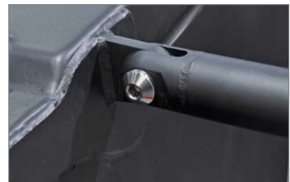
Polished Spud Bolt shown at forward strut firewall mount.
