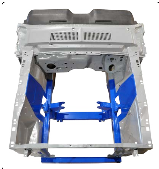
Gray Area: Unmodified stock sheet metal Blue Area: Subframe assembly and tower delete panels
