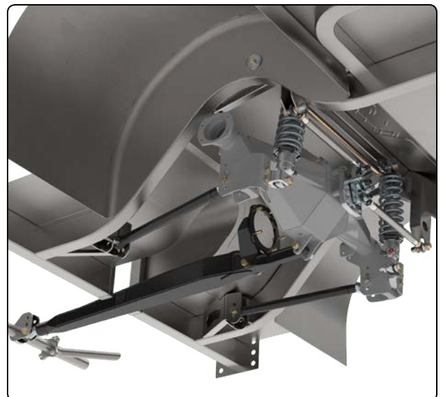
A Watts-link with roll-center height adjustment is used for superior lateral location and suspension tuning.
