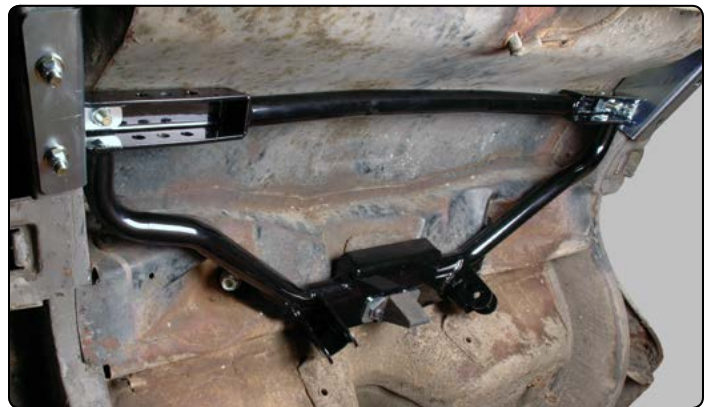
"Self-positioning" uses pinion snubber and top shock mount holes.
