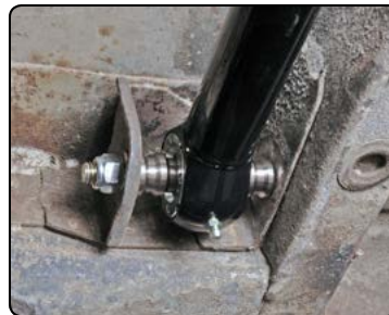
Lower links use leaf-spring brackets.
