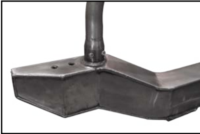
Frame Gemini Connector welds easily to front frame rail.
