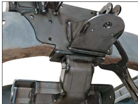
Upper suspension mount sits outside the frame and between the lower crossmember and frame.
