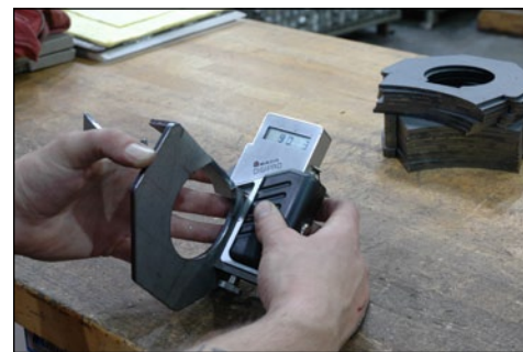
▲ Each part is QA checked using measurement devices or a physical-fit gauge. Any variances will be corrected before moving on to welding.
