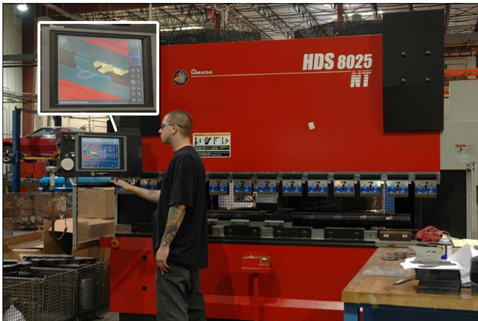
▲ After the individual FAB9™ components have been laser-cut they must be bent on Chassisworks CNC Amada HDS press brake. This piece of equipment allows the original computer model to be bent into an exact replica of the intended design.
