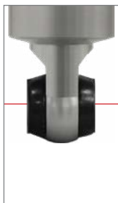
EYES AND THROUGHBOLTS Measure to center of shock eye, sleeve, or cantilever pin.
