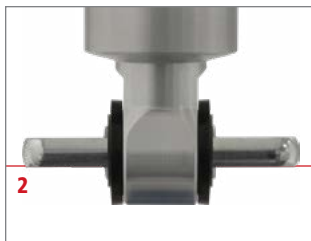
1-PIECE CROSSBARS AND 2-PIECE CROSSBARS Measure to side of crossbar that contacts shock mounting surface.
