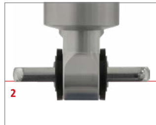
1-PIECE CROSSBARS AND 2-PIECE CROSSBARS Measure to side of crossbar that contacts shock mounting surface.
