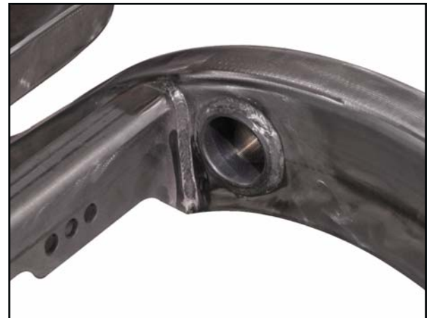
Anti-roll bar mounting sleeves are welded into the frame rail positioning the bar close to the undercarriage and clear of suspension and exhaust.
