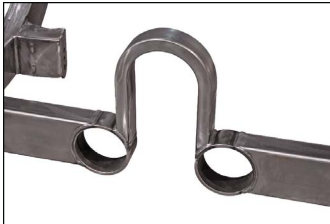
Tall driveshaft loop allows body to sit lower over the drivetrain without risk of driveshaft contact. Crossmember features factory-welded, dual 4" ID exhaust ports.
