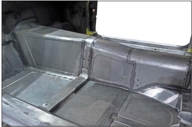
Installed lowered-seat-mount assembly shown with prefabricated front floor, transmission tunnel, driveshaft tunnel, and rear floor.
