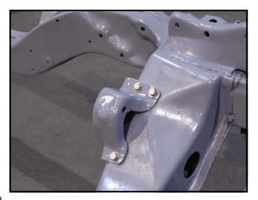
The new billet motor mount adapters will use the factory holes in the subframe. The driver-side adapter has the round hole for the billet mount. The passenger side adapter has a slotted hole.
