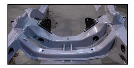
Once the billet motor mounts are attached to the engine they will slide into the adapters and be secured with the 1/2" hardware included with the mounts. Shown is the LS style billet mount.
