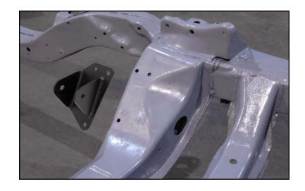
3. Bolt the driver side billet motor plate adapter to the subframe with the 3/8-16 x 1-1-/4" socket-head cap screws, flat washers and locknuts supplied. Place a flat washer under the head of the cap screw and before the locknut. Tighten all fasteners and torque to 25 lb-ft.
