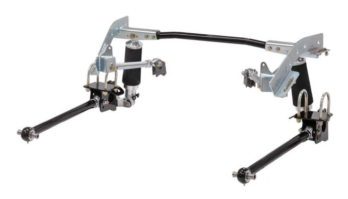
**Description:** Canted 4-bar rear air suspension for 1968-1974 Nova. Includes upper links, lower links, suspension cradle, axle brackets, and VariShock ShockWaves.
