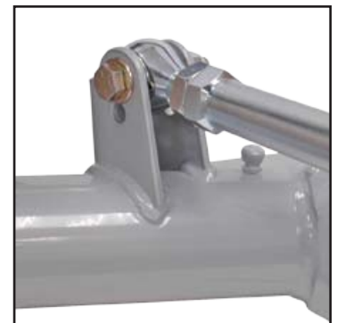
Accurate weld-fixture placement.
