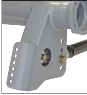
4-position FAB9™ lower arm bracket
