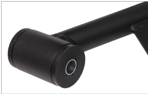
Fluted premium-urethane bushings for improved grease retention and reduced friction.
