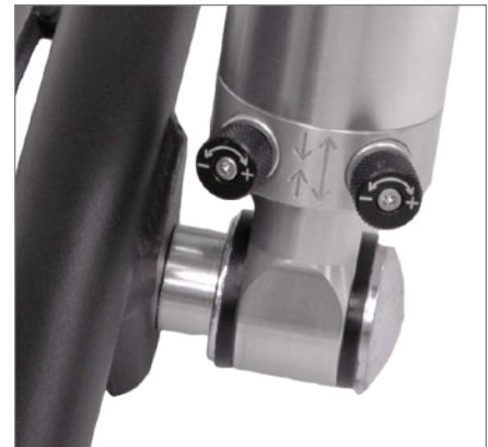
Gusseted lower shock mount with specialized hardware for more tire clearance.
