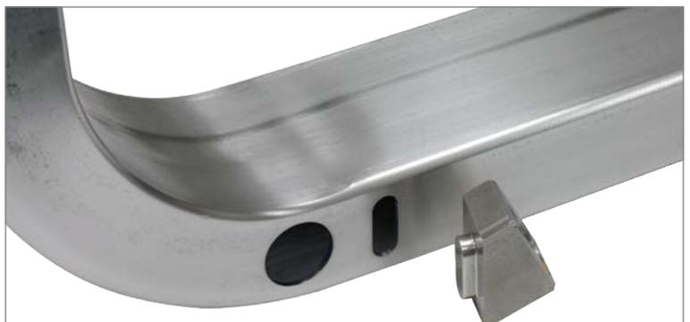
Billet rack-and-pinion mount inserts into machined slot on crossmember.
