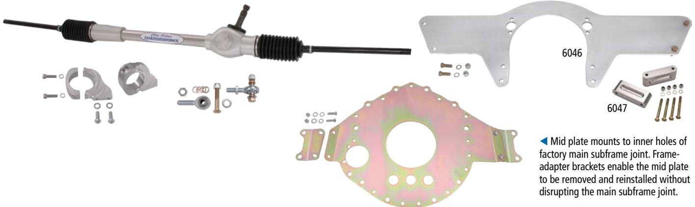
◀ Mid plate mounts to inner holes of factory main subframe joint. Frame-adapter brackets enable the mid plate to be removed and reinstalled without disrupting the main subframe joint.
