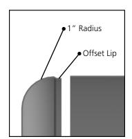
Offset tub-cap lip seats underneath edge of tub skin, creating an easy to align overlap joint with flush outer surface.
