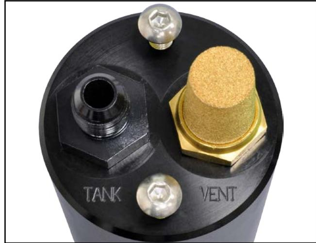
The canister base features the two mounting screws as well as o-ringed ports for -6 hose attachment and the -8 sintered vent. Each port is clearly labeled.
