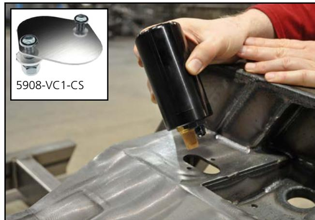
Chassisworks gStreet IRS rear frame comes pre-drilled for vented canister installation; drill jig template also available. Stainless cover plate available if the hole is unused.
