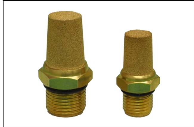
A large -8 sized sintered bronze breather vent is used instead of the more commonly found -6 size. The increased surface area and port volume improves vent flow without increasing air velocity.
