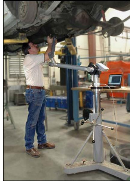
The FaroArm is used to digitally scan multiple vehicles and create an exact computer model for development.
