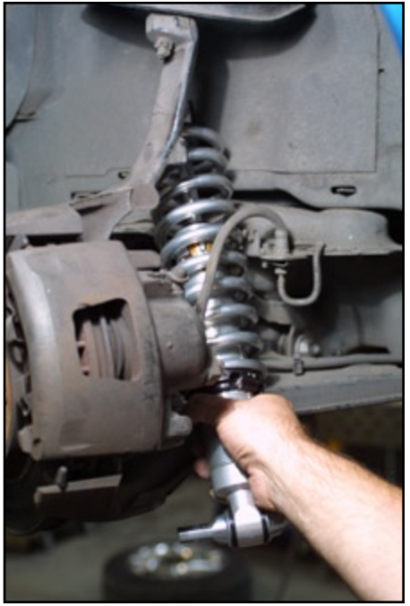
Installing the coil-over assembly.
