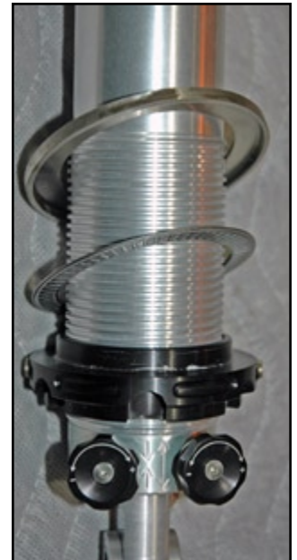
Grease the roller bearings and then, install the coil spring bearing on the lower spring seat as shown.
