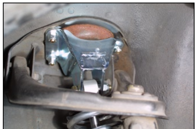
Upper mount with coil-over assembly bolted in.
