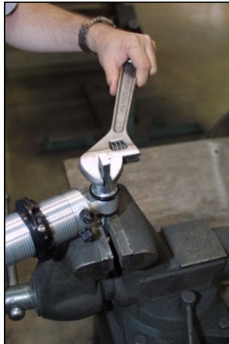
Installing lower crossbar and urethane bushings.
