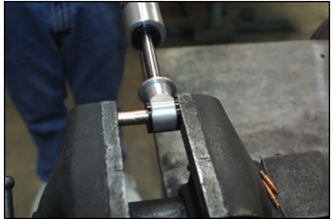
Installing upper urethane bushings and steel sleeve.
