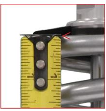
Hook the tape measure against the spring at the upper spring seat slot.
