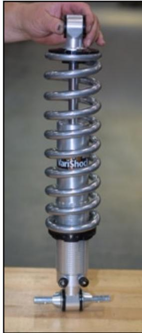
Coil-over and spring assembly ready to install.
