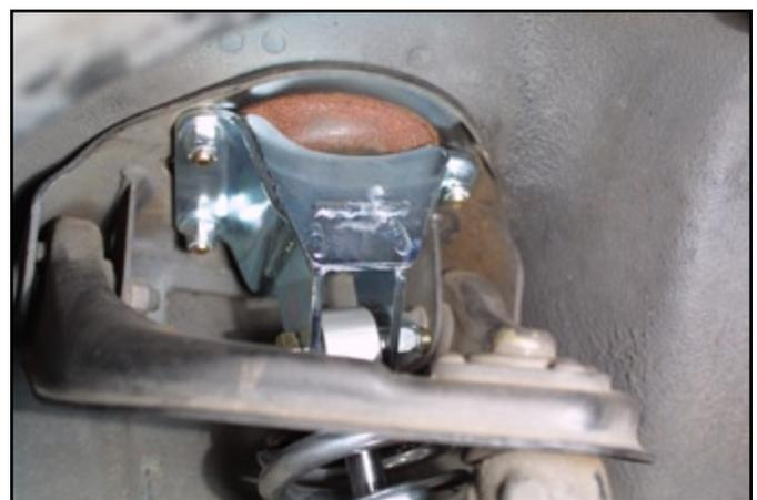
Upper mount with coil-over assembly bolted in.
