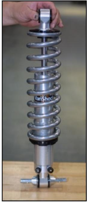
Coil-over and spring assembly ready to install.
