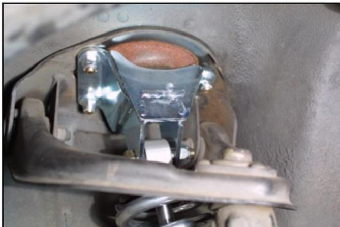
Upper mount with coil-over assembly bolted in.
