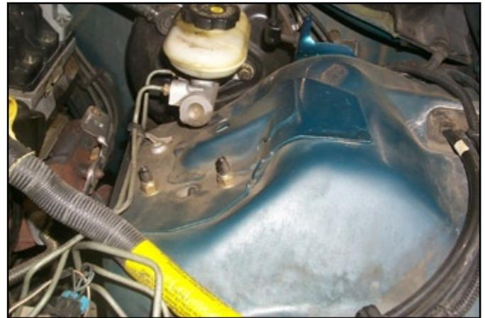
Here you can see the OEM mounting bolts & studs. Move the master cylinder toward the engine to make removing the rear bolts easier.
