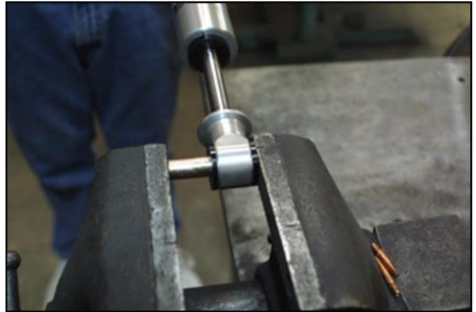
Installing upper urethane bushings and steel sleeve.
