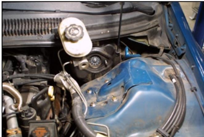
Here the master cylinder has been moved and the new bolts are installed to secure the new upper coil-over mounting bracket.
