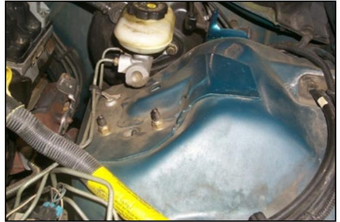
Here you can see the OEM mounting bolts & studs. Move the master cylinder toward the engine to make removing the rear bolts easier.
