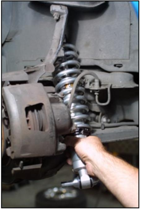
Installing the coil-over assembly.
