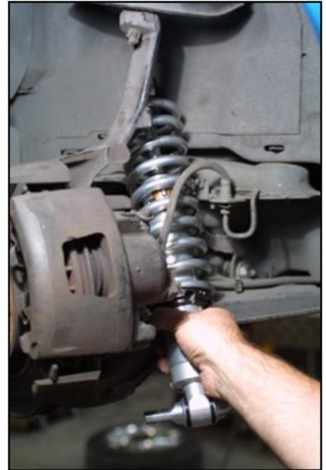
Installing the coil-over assembly.
