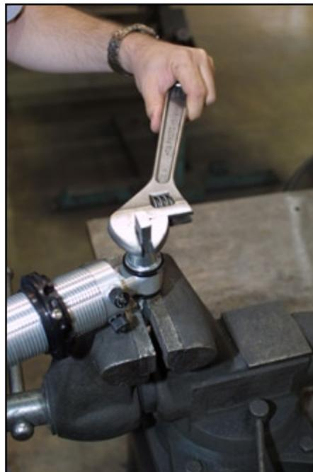
Installing lower crossbar and urethane bushings.
