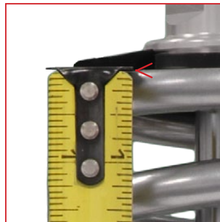
Hook the tape measure against the spring at the upper spring seat slot.
