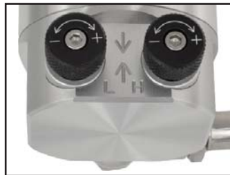
Bump (Compression) Located on remote reservoir
