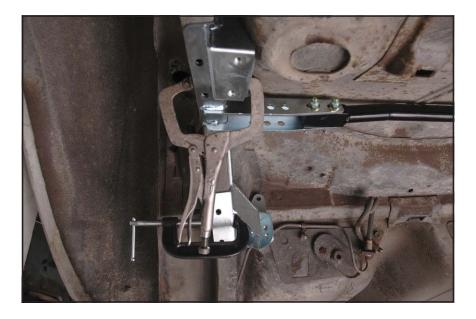
26. Unclamp the frame brackets but DO NOT loosen or remove the 3/8" upper-crossmember hardware at the frame brackets. Try not to bump the brackets from their correctly fit position. Lower the cradle assembly and set aside.
