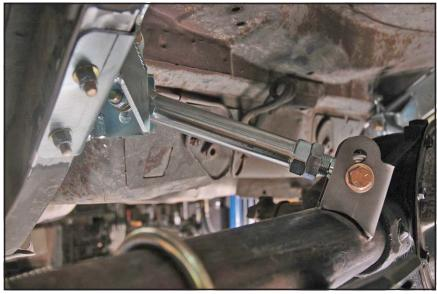
57. Install the lower-shock mounts at the lower axle bracket using 3/8" hardware. Leave one blank hole below the mount for initial setup.
