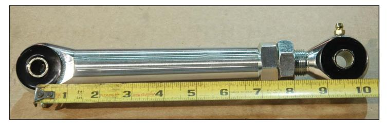
55. Attach the non-adjustable end of upper links to the upper holes of the cradle with 1/2" bolts, flat washers and locknuts. Grease zerk must point down.
