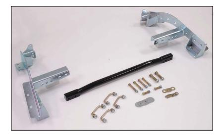
8. Prepare frame rail brackets for welding to chassis (performed in a later step). Use disc sander with a fine grit pad to remove zinc coating along outside edges where the welds will be made. The zinc inside the larger holes can be removed with die grinder.
