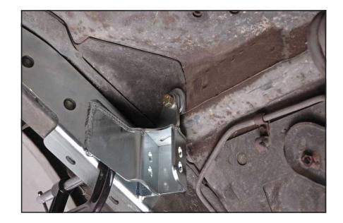
35. Verify the shock bracket channel edge is the same distance from the flat vertical section of the undercarriage. Ours measured 10-1/2".
