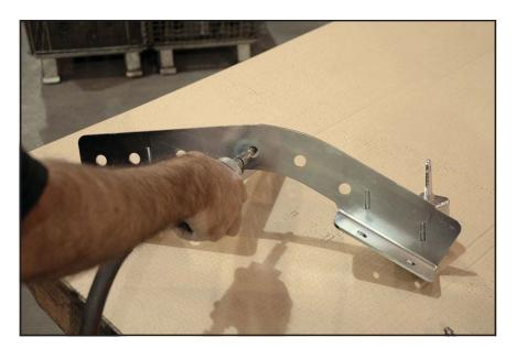
9. Bolt the driver and passenger frame brackets to the shock crossmember mounting blocks with the 3/8" bolts, flat washers and locknuts center in the slots.
