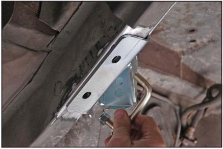
39. Once all the locknuts are in place, begin tightening each nut until it contacts the bracket. The u-bolt must "snugged-up" into a level, settled position before final tightening.
