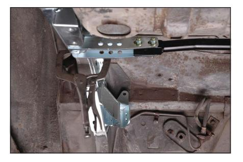
34. Place the correct amount of shims between the tab and the floor. Install and torque 3/8" forward mount tab hardware to 35 lb-ft.
