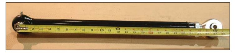
51. Install the lower suspension links at the factory front leaf spring mount using 1/2" diameter bolts, flat washers, and locknuts. Grease zerk fittings must point downward. The bolts must be installed from the direction shown in the photo to allow clearance for the locking nut once on the vehicle. Torque to 65 lb-ft.
