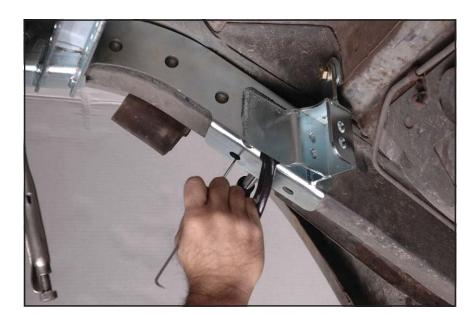
24. Use a 3/8"-diameter bit to drill a starting hole through the factory frame rail <u>at each of the eight</u> oval holes along the bottom of the frame rail ONLY. These holes will be opened up in a later step. The clamped cradle brackets will help to correctly guide the drill.
