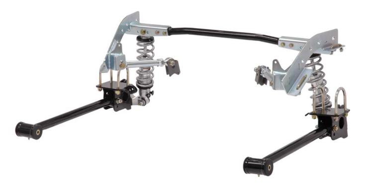
**Description:** Canted 4-bar coil-over rear suspension for 1967-1969 Camaro and Firebird. Includes upper links, lower links, suspension cradle, axle brackets, shocks and springs
