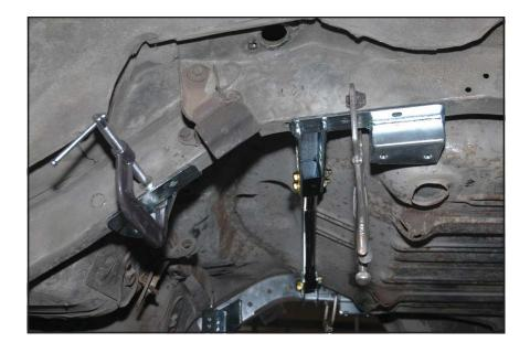
22. Make sure the 3/8" upper crossmember mounting hardware is tight before marking the undercarriage.
