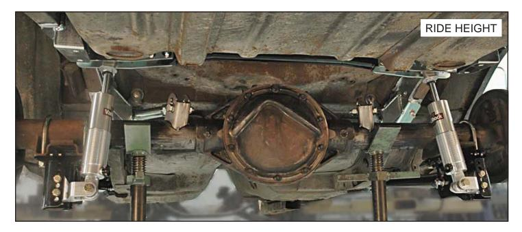
71. Using a jack, cycle the rear suspension through its full range of vertical travel and body roll in both directions to check for binding and potential clearance issues at all suspension joints and along the lengths of any moving parts including the rearend housing.
