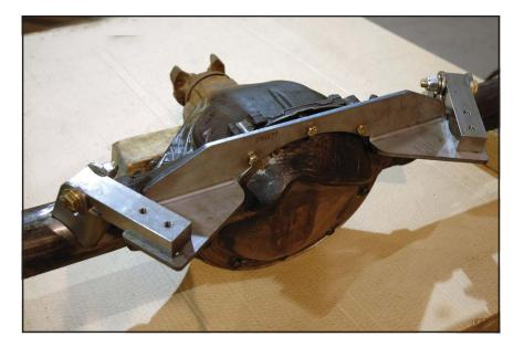
47. When leaving the rearend cover on the housings use the provided spacers. Also make sure the bracket bosses are at the forward holes. If welding with the cover removed the spacers are NOT used and the bracket bosses are mounted in the rear holes. Only tack weld the brackets at this time.
