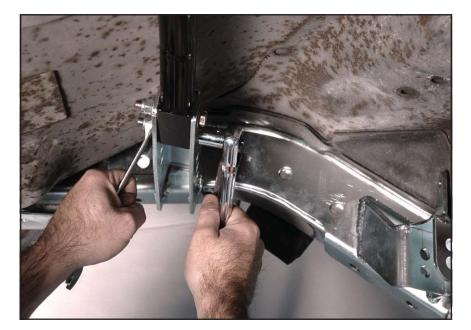
23. Clearly mark the weld-prep areas onto the undercarriage by scribing guidelines onto the surface of the frame rail. Scribe the overall outline of the bracket, the holes along the inside of the frame rail, and finally the eight oval holes along the bottom of the frame rail.
