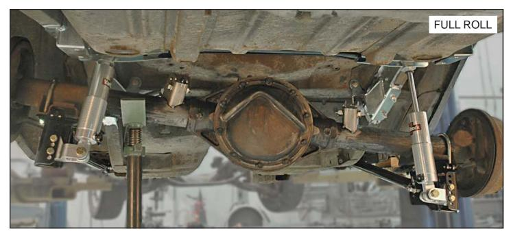
72. Once clearance has been verified, remove the housing and final weld the upper link brackets to the housing.
