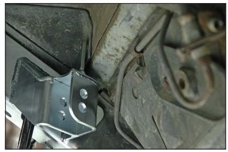
Place the flat washer over the 3/8-24 x 1-3/4" hex bolt and insert through the forward mount tabs, shims, and through the floor behind the seat.
