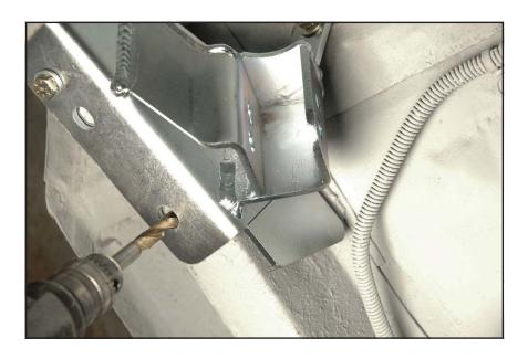
25. After all weld-prep areas are marked and starting holes drilled, remove the mounting hardware at the forward mounting tabs.
