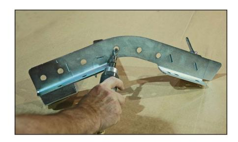
9. Bolt the driver and passenger frame brackets to the shock crossmember mounting blocks with the 3/8" bolts, flat washers and locknuts center in the slots.
