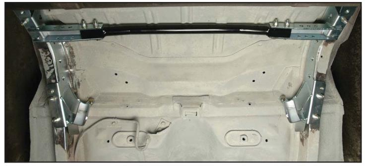
42. Tack weld each bracket to the frame rail, and then stitch weld along the longer seam lengths. The seams at the forward end of the brackets should be completely welded with the bead extending 1" past the corner. Rosette weld around the holes on the inside of the frame rail, being careful not to burn through the frame rail. Use the photo below as a guide.
