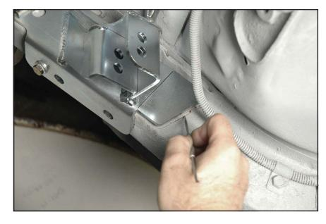
24. Use a 3/8"-diameter bit to drill a starting hole through the factory frame rail at each of the eight oval holes along the bottom of the frame rail ONLY. These holes will be opened up in a later step. The clamped cradle brackets will help to correctly guide the drill.
