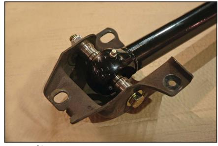
53. Use the factory bolts to install the front spring hanger into the frame.
