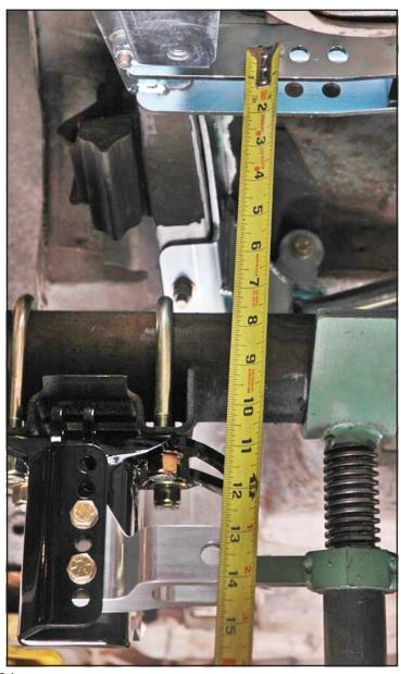
65. The upper suspension links can now be used to center the rearend in relation to the chassis, and then to adjust pinion angle. Link ends will need to be unbolted from axle brackets to adjust length. One full turn IN on one link and OUT on the other link will move the rearend housing approximately 3/16" toward the shortened side. Measuring from a point on the frame to the end of the axle on each side is the best way to center the housing in the car.
