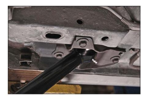
54. Position the rearend housing under the car on jack stands. Attach the lower suspension links to the axle brackets with 1/2" bolts, flat washers, and locknuts. Use the second hole from the bottom on the axle brackets for initial installation. Torque to 65 lb-ft.
