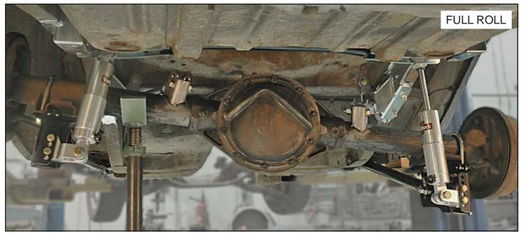
73. Once clearance has been verified, remove the housing and final weld the upper link brackets to the housing.
