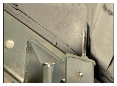
18. Place the flat washer over the 3/8-24 x 1-3/4" hex bolt and insert through the forward mount tabs, shims, and through the floor behind the seat.
