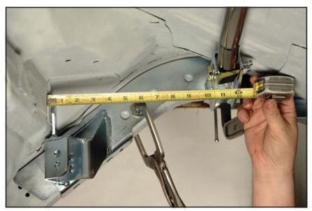
36. On one end of each squarecorner u-bolt, install a 3/8" flat washer and locknut. DO NOT SKIP THIS STEP. It is possible to lose the u-bolt inside of the frame rail.
