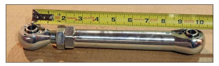
56. Attach the non-adjustable end of upper links to the upper holes of the cradle with 1/2" bolts, flat washers and locknuts. Grease zerk must point down.
