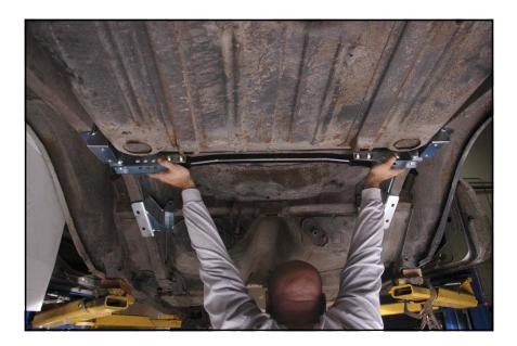
27. Use a die grinder, grinding-cone drill attachment, or file to enlarge the oval holes up to the scribe marks on the frame rails.
