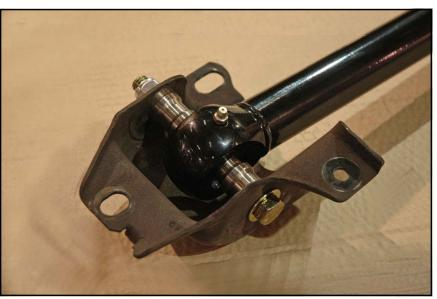
52. Use the factory bolts to install the front spring hanger into the frame.
