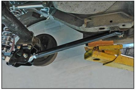
54. Adjust upper suspension links to 9-1/2" center to center of the mounting holes.
