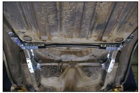
42. Tack weld each bracket to the frame rail, and then stitch weld along the longer seam lengths. The seams at the forward end of the brackets should be completely welded with the bead extending 1" past the corner. Rosette weld around the holes on the inside of the frame rail, being careful not to burn through the frame rail. Use the photo below as a guide.
