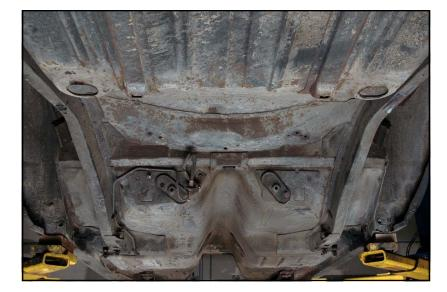
7. The two frame brackets, upper shock crossmember, and hardware make up the cradle assembly.
