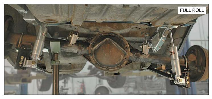
71. Once clearance has been verified, remove the housing and final weld the upper link brackets to the housing.
