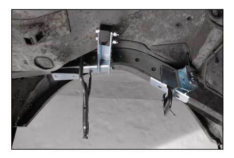
11. Ensure the cradle is positioned square to the chassis. On the driver side and passenger side, measure from the flat vertical section of undercarriage sheet metal to the lowest corner of the shock mount. Our vehicle measured 10-1/2". Your measurement may differ slightly. <u>Record this measurement.</u> Measurements should be equal from one side of the vehicle to the other.
