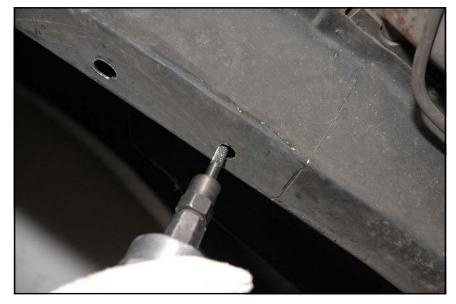
28. Use a scotch-brite disc pad or wire-brush drill attachment to expose bare metal along the weld areas marked on the frame rail earlier.
