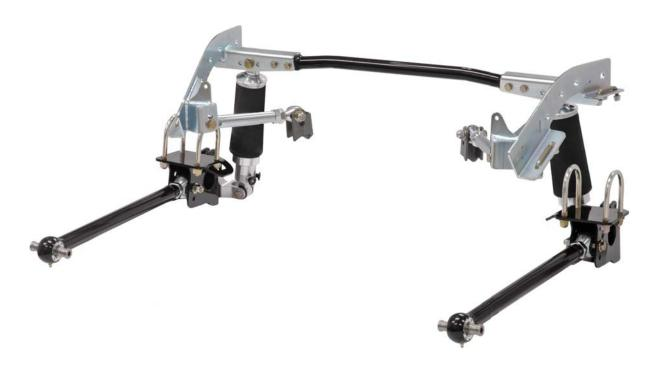
**Description:** Canted 4-bar rear air suspension for 1967-1969 Camaro and Firebird. Includes upper links, lower links, suspension cradle, axle brackets, and VariShock air-spring shocks.
