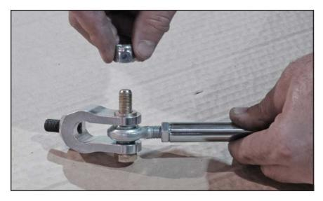
15. Slide each clevis over the end of the anti-roll bar until the set screw lines up with the first detent.Tighten the set screw and then the locknut. This is the baseline position for anti-roll bar and provides the softest setting.
