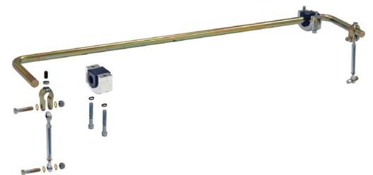
**Description:** Sliding-link anti-roll bar for 1967-1969 Camaro/Firebird g-Bar rear suspension. **Includes:** 5/8"-diameter anti-roll bar, billet clevis, endlink assemblies, and billet mounts. **Notes:** Frame mount is part of g-Bar frame bracket weldment and ships with g-Bar suspension system. Installation of g-Bar frame brackets requires welding.
