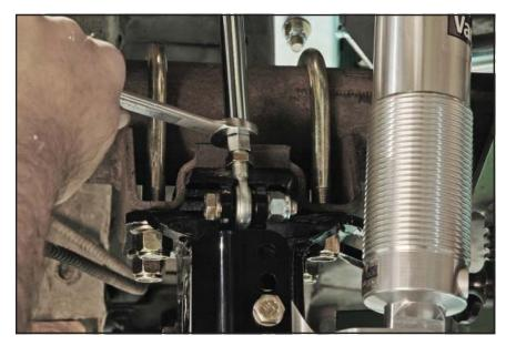
19. Check for any clearance issue with the anti-roll bar throughout the suspension's range of travel. This must be done without springs installed on the shocks or without air pressure if using ShockWaves®.
