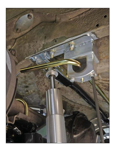
9. Measure from each billet housing to the outside of the bar on each side to verify that the anti-roll bar is centered.
