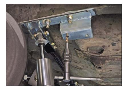
Secure bushing mounts with 3/8"-16 x 2-1/2" socket head cap screws and high-collar lock washers. Fasteners will feel tight as they are screwed in due to crimped weld locknuts in cradle frame brackets. Torque fasteners to 30 lb-ft.
