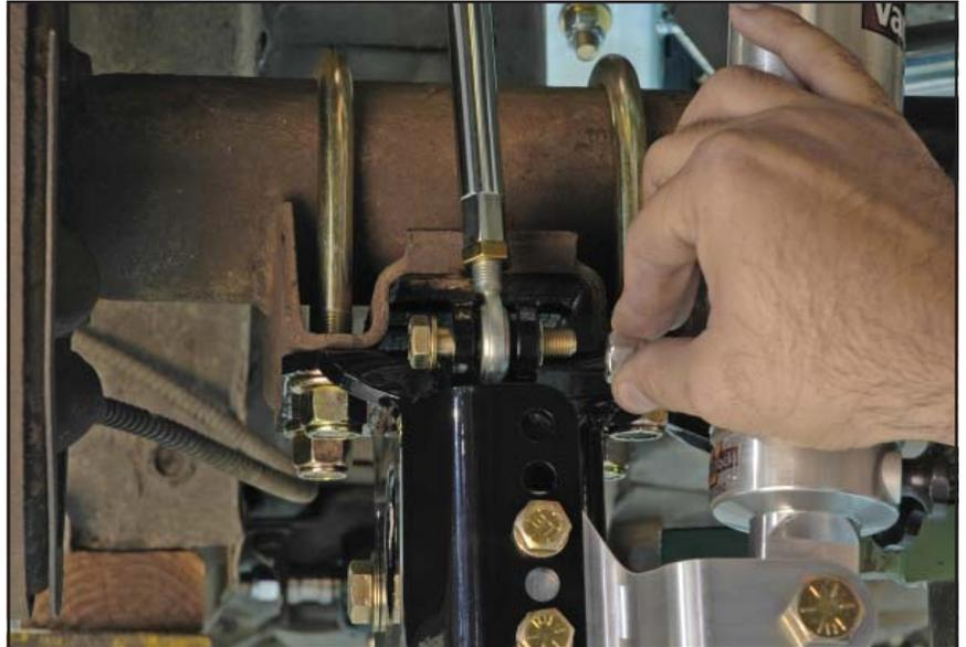
17. Adjuster links should be in a neutral position, meaning that there is NO preload placed upon the anti-roll bar. If there is any preload present, adjuster links will be difficult to turn by hand. If necessary, adjust one of the link assemblies to a shorter length until preload is neutral. Do NOT add preload to chassis using adjuster links.
