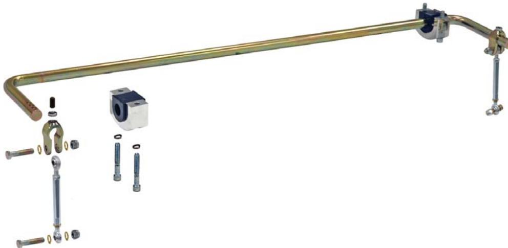
**Description:** Sliding-link anti-roll bar for 1970-1981 Camaro/Firebird g-Bar rear suspension.
