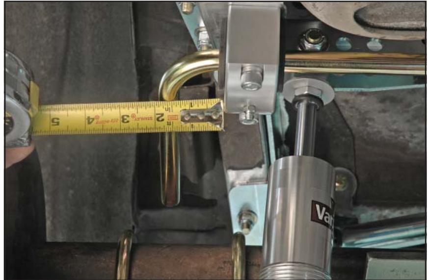
10. Thread the 3/8" jam nuts on to the male rod ends, leaving 5 to 7 threads showing between the jam nut and rod end body.
