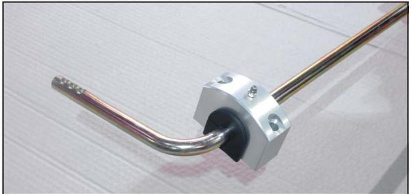
5. Rotate the bushing housing to its correct orientation. The open end of the housing and detents on the anti-roll bar must both face up.
