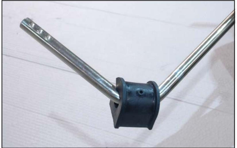
3. Install a zerk fitting into each billet bushing housing.
