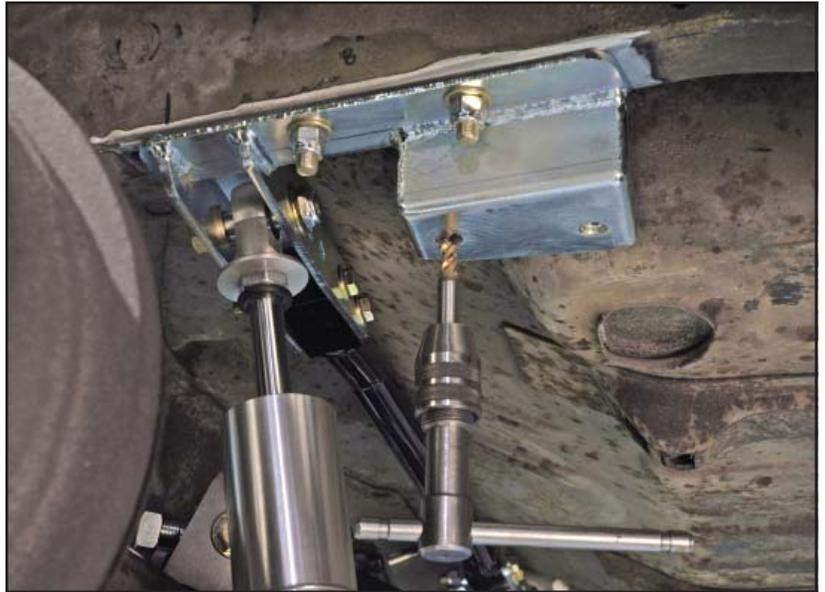
8. Secure bushing mounts with 3/8"-16 x 2-1/2" socket head cap screws and high-collar lock washers. Fasteners will feel tight as they are screwed in due to crimped weld locknuts in cradle frame brackets. Torque fasteners to 30 lb-ft.
