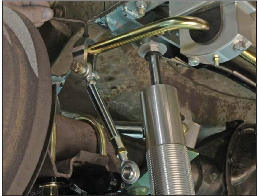
16. Bolt the opposite end of each adjuster endlink assembly to the tabs on the lower axle brackets, using 3/8-24 x 1-3/4" hex bolts, aircraft washers and locknuts.
