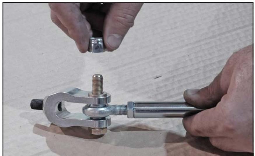
15. Slide each clevis over the end of the anti-roll bar until the set screw lines up with the first detent. Tighten the set screw and then the locknut. This is the baseline position for anti-roll bar and provides the softest setting.
