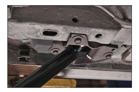
53. Position the rearend housing under the car on jack stands. Attach the lower suspension links to the axle brackets with 1/2" bolts, flat washers, and locknuts. Use the second hole from the bottom on the axle brackets for initial installation. Torque to 65 lb-ft.
