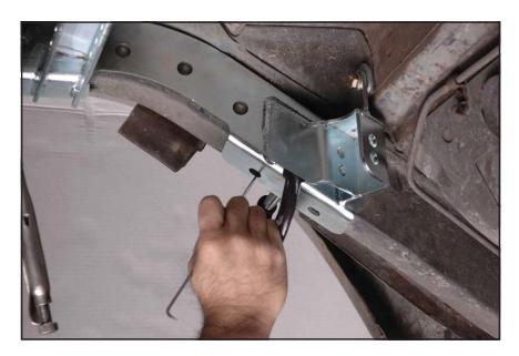
24. Use a 3/8"-diameter bit to drill a starting hole through the factory frame rail at each of the eight oval holes along the bottom of the frame rail ONLY. These holes will be opened up in a later step. The clamped cradle brackets will help to correctly guide the drill.
