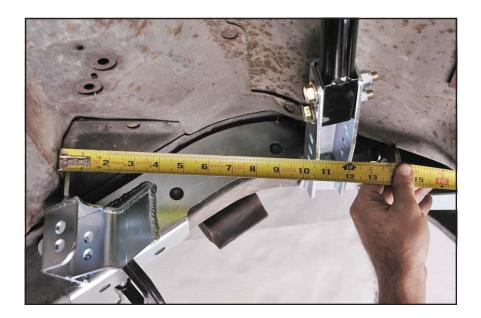
16. At each forward mount tab, drill a 3/8" diameter hole through the triple-layer floor panel behind the rear seat, using the forward mounts tab as a guide.
