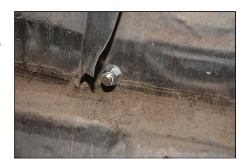
20. Tighten the forward mount tab bolts to hold the cradle in place. Do not torque to final specs at this time.
