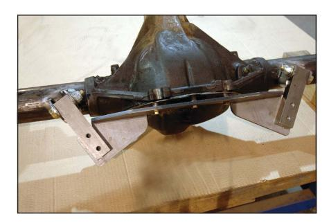
48. Use a 1/2" diameter drill bit to enlarge the holes in the factory spring plates for the u-bolts.
