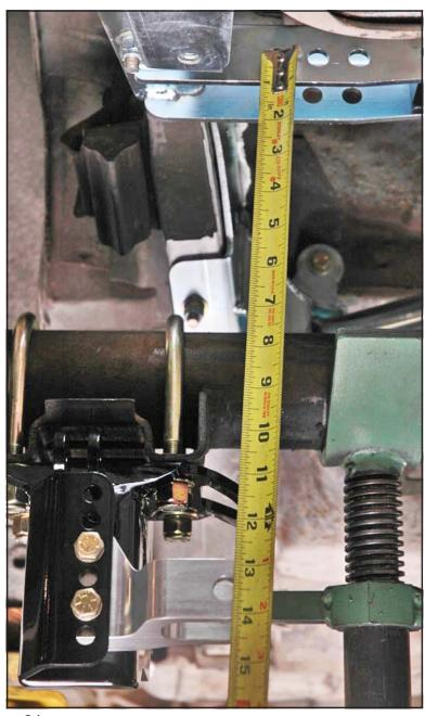
64. The upper suspension links can now be used to center the rearend in relation to the chassis, and then to adjust pinion angle. Link ends will need to be unbolted from axle brackets to adjust length. One full turn IN on one link and OUT on the other link will move the rearend housing approximately 3/16" toward the shortened side. Measuring from a point on the frame to the end of the axle on each side is the best way to center the housing in the car.
