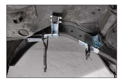
11. Ensure the cradle is positioned square to the chassis. On the driver side and passenger side, measure from the flat vertical section of undercarriage sheet metal to the lowest corner of the shock mount. Our vehicle measured 10-1/2". Your measurement may differ slightly. Record this measurement.
