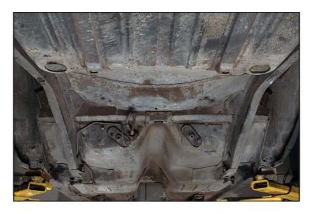
7. The two frame brackets, upper shock crossmember, and hardware make up the cradle assembly.
