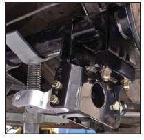
Shock Extenders (P/N: 300-0163 or 300-0164) Use with bolt-on or weld-on
