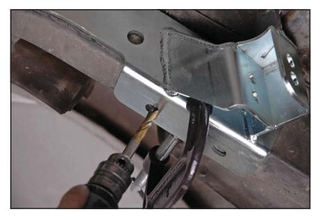
25. After all weld-prep areas are marked and starting holes drilled, remove the mounting hardware at the forward mounting tabs.
