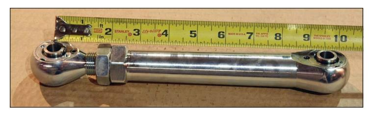
55. Attach the non-adjustable end of upper links to the upper holes of the cradle with 1/2" bolts, flat washers and locknuts. Grease zerk must point down.
