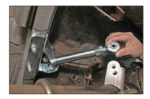
56. Bolt opposite end of each upper link to the lower hole at the axle bracket. Grease zerk must point up.
